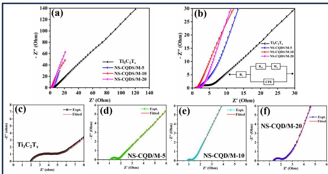
**Fig. 9** (a) Nyquist plots of pristine Ti<sub>3</sub>C<sub>2</sub>T<sub>x</sub> along with the three composites, (b) high-frequency portion of Nyquist plots, and the fitted high-frequency part of Nyquist plots of (c) pristine Ti<sub>3</sub>C<sub>2</sub>T<sub>x</sub>, (d) NS-CQD/M-5, (e) NS-CQD/M-10, and (f) NS-CQD/M-20.
