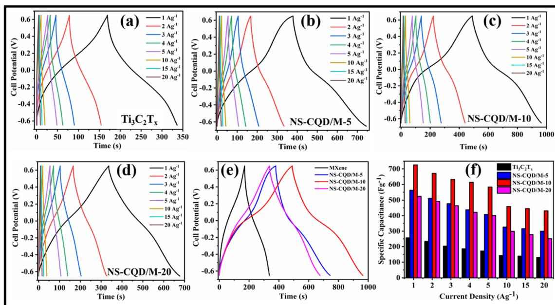
**Fig. 7** GCD curves of (a) Ti<sub>3</sub>C<sub>2</sub>T<sub>x</sub>, (b) NS-CQD/M-5, (c) NS-CQD/M-10, (d) NS-CQD/M-20, (e) all the composites in comparison with pristine Ti<sub>3</sub>C<sub>2</sub>T<sub>x</sub> at a fixed current density of 1 A g<sup>-1</sup>, and (f) comparison of specific capacitances of all the composites at varying current densities.
