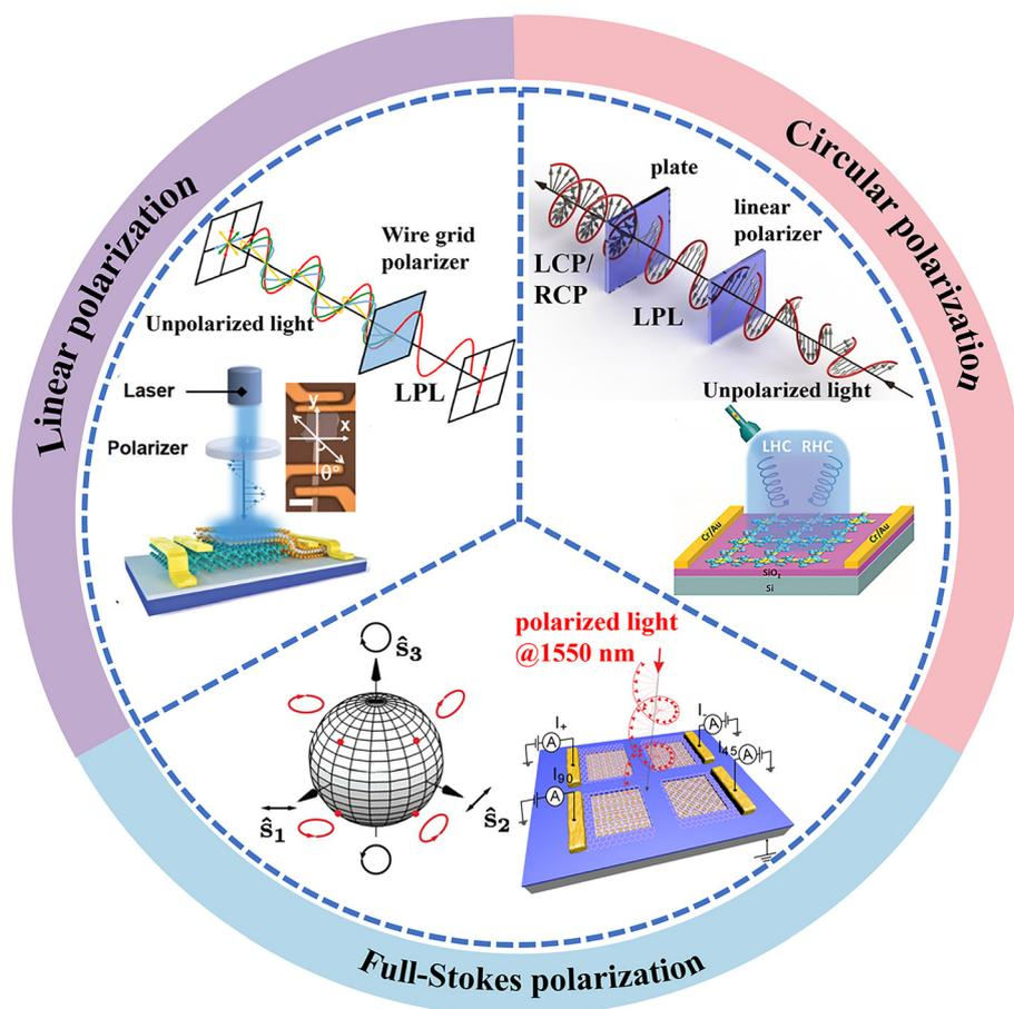
**Fig. 1** The main classifications of polarization-sensitive photodetectors: linear-,<sup>17</sup> (copyright 2021, Royal Society of Chemistry) circular-,<sup>18</sup> (copyright 2023, John Wiley and Sons) and full-Stokes polarization<sup>19,20</sup> (copyright 2016, Optica Publishing Group and copyright 2020, American Chemical Society).
