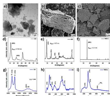
**Fig. 1** Morphological and structural characterization of the initial (a, d and g) GO, (b, e and h) MX and (c, f and i) TMDC nano-materials by (a–c) electron microscopy, (d–f) X-ray diffraction and (g–i) Raman spectroscopy, respectively.
