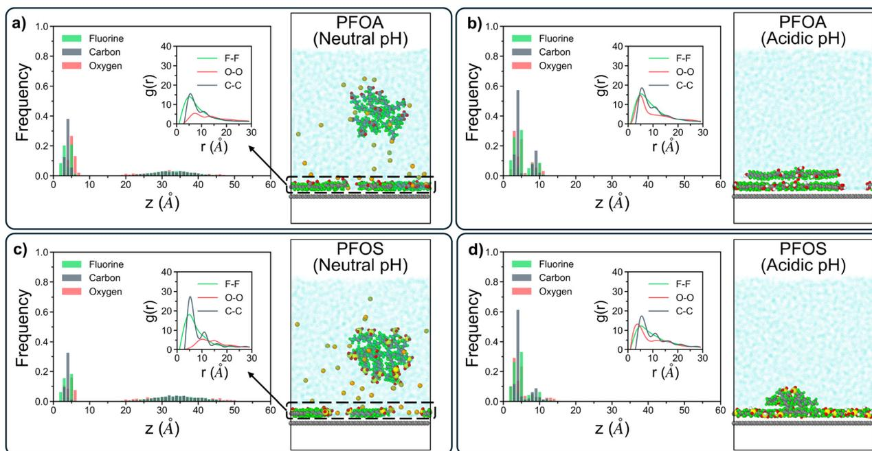
**Fig. 2** Linear density profiles and radial distribution function plots with accompanying simulation snapshots for (a) PFOA at neutral pH, (b) PFOA at acidic pH, (c) PFOS at neutral pH, and (d) PFOS at acidic pH. For each plot, the radial distribution function only accounts for the adsorbed PFAS, excluding PFAS in solution.
