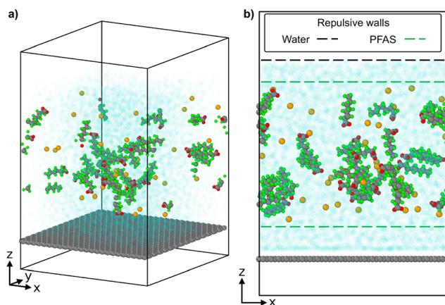
Fig. 1 A representative (a) isotropic snapshot of the pre-equilibrated simulations and (b) front view with repulsive walls highlighted.
