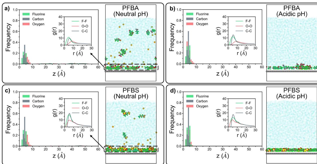
**Fig. 3** Linear density profiles and radial distribution function plots with accompanying simulation snapshots for (a) PFBA at neutral pH, (b) PFBA at acidic pH, (c) PFBS at neutral pH, and (d) PFBS at acidic pH. For each plot, the radial distribution function only accounts for the adsorbed PFAS, excluding PFAS in solution.
