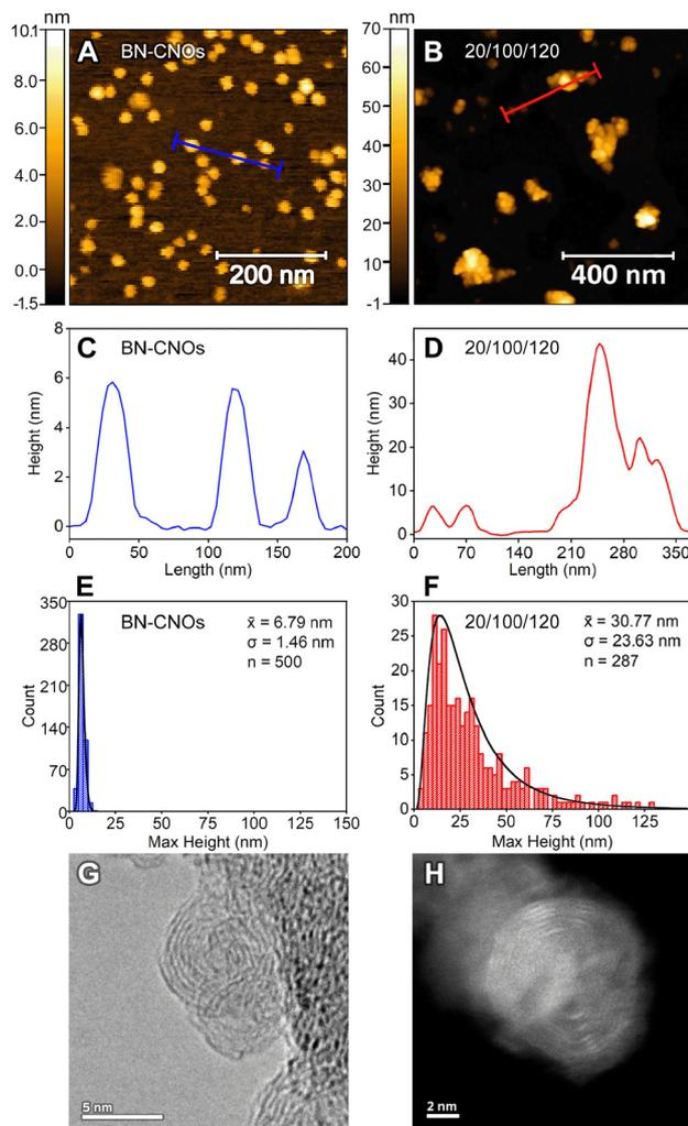
**Fig. 2** AFM, HRTEM and HAADF-STEM studies|AFM micrograph of (A) BN-CNOs and (B) 20/100/120 wt% HA-DMPE/BN-CNO/DOX; their respective line profiles (C & D); and their respective size distributions (E & F). Electron microscopy studies depicting a HRTEM image of BN-CNOs (G), and a HAADF-STEM image of the 20/100/120 wt% HA-DMPE/BN-CNO/DOX formulation (H).
