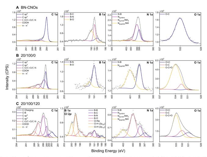
Fig. 1 XPS studies | High-resolution core level XPS spectra of (A) BN-CNOs (top row; C 1s, B 1s, N 1s, and O 1s); (B) the 20/100/0 wt% HA-DMPE/ BN-CNO/DOX formulation (middle row; C 1s, B 1s, N 1s, and O 1s); and of (C) the 20/100/120 wt% HA-DMPE/BN-CNO/DOX formulation (bottom row; C 1s, B 1s & Cl 2p, N 1s, and O 1s). Spectra include experimental data (grey, scatter) and the fitted peak deconvolution envelope (grey, line).
