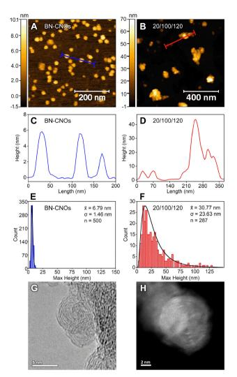
Fig. 2 AFM, HRTEM and HAADF-STEM studies AFM micrograph of (A) BN-CNOs and (B) 20/100/120 wt% HA-DMPE/BN-CNO/DOX; their respective line profiles (C & D); and their respective size distributions (E & F). Electron microscopy studies depicting a HRTEM image of BN-CNOs (G), and a HAADF-STEM image of the 20/100/120 wt% HA-DMPE/BN-CNO/DOX formulation (H).
