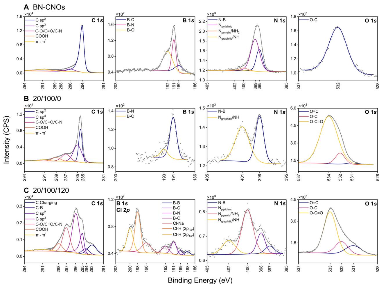
**Fig. 1** XPS studies | High-resolution core level XPS spectra of (A) BN-CNOs (top row; C 1s, B 1s, N 1s, and O 1s); (B) the 20/100/0 wt% HA-DMPE/BN-CNO/DOX formulation (middle row; C 1s, B 1s, N 1s, and O 1s); and of (C) the 20/100/120 wt% HA-DMPE/BN-CNO/DOX formulation (bottom row; C 1s, B 1s & Cl 2p, N 1s, and O 1s). Spectra include experimental data (grey, scatter) and the fitted peak deconvolution envelope (grey, line).
