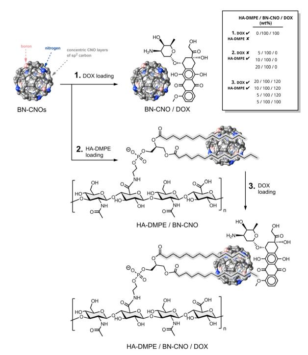
Scheme 1 Nanocarrier preparation|(1) DOX-loading of BN-CNOs to prepare the HA-DMPE-free BN-CNO/DOX; (2) HA-DMPE-loading of BN-CNOs to prepare the DOX-free HA-DMPE/BN-CNOs; and (3) the subsequent DOX-loading of HA-DMPE/BN-CNOs to prepare HA-DMPE/BN-CNO/DOX. All wt% ratios of the BN-CNO-based nanocarriers formulated and investigated in this study are tabulated in the inset. Procedures and experimental conditions for the loading processes are detailed in the Materials and Methods section.
