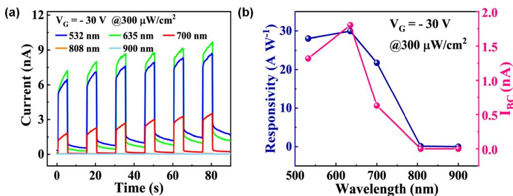
Fig. 5 Phototransistor metrics. (a) Photocurrent of the MoS<sub>2</sub> phototransistor at different wavelengths. (b) Response and  $I_{BC}$  with wavelength at a gate voltage of  $-30$  V and an optical power of  $300 \mu\text{W cm}^{-2}$ .
