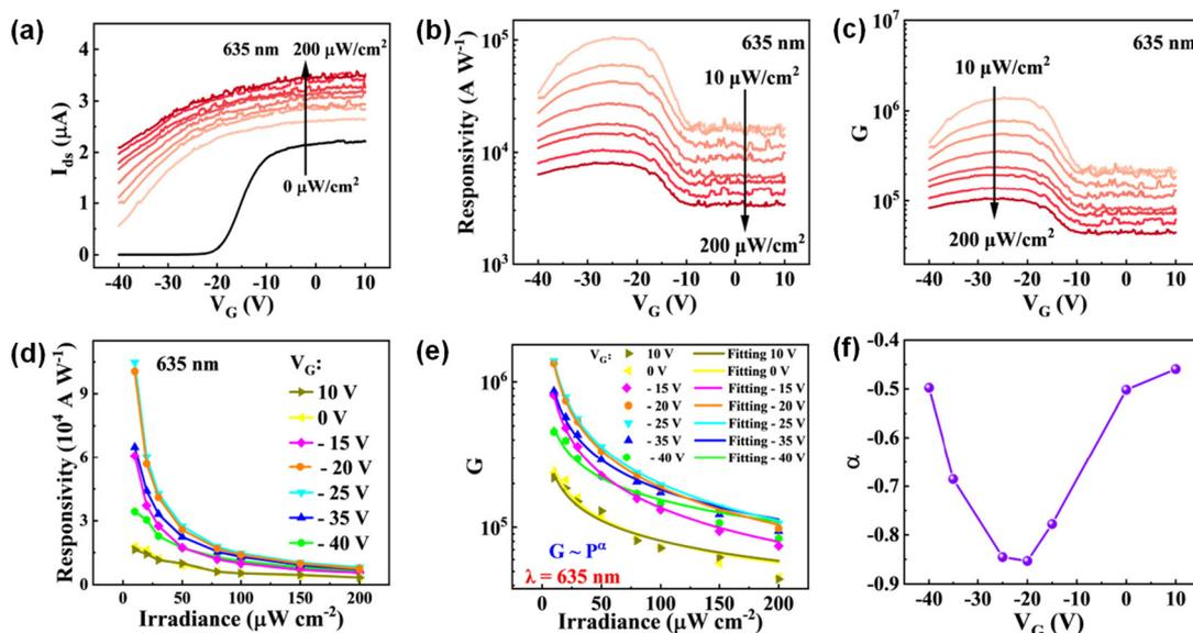
**Fig. 2** Optoelectronic response and fitting. (a) Transfer characterization, (b) responsivity and (c) photo gain of the MoS<sub>2</sub> phototransistor under illumination. (d) Optical responsivity and (e) gain of the device *versus* the optical power density at different gate voltages. The solid line in (e) is the fitted curve of gain and optical power. (f)  $\alpha$ – $V_G$  curve.
