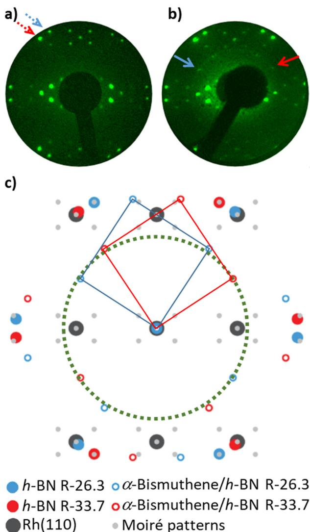
**Fig. 3** Relative orientation between the  $\alpha$ -bismuthene lattice and the h-BN/Rh(110) support underneath. (a) LEED pattern representative of the as-grown h-BN/Rh(110) surfaces; (b) LEED pattern acquired after  $\alpha$ -bismuthene growth on h-BN/Rh(110); (c) schematics illustrating the origin of the different diffraction features observed in the LEED pattern shown in panel (b). Electron energy (a) and (b) 40 eV.
