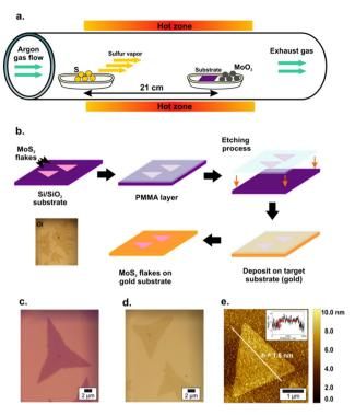
Fig. 1 (a) Schematic representation of the atmospheric pressure CVD setup with a one-zone furnace used to grow the MoS2 structures. (b) Illustration of the PMMA-assisted method to transfer the MoS<sub>2</sub> flakes to a gold substrate. Optical images (c) before and (d) after the transferring process. (e) AFM image for the MoS<sub>2</sub> flakes and their cross-section to determine the approximate thickness.
