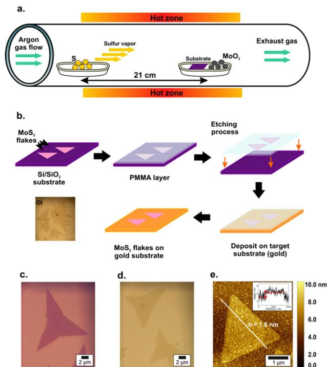
**Fig. 1** (a) Schematic representation of the atmospheric pressure CVD setup with a one-zone furnace used to grow the MoS<sub>2</sub> structures. (b) Illustration of the PMMA-assisted method to transfer the MoS<sub>2</sub> flakes to a gold substrate. Optical images (c) before and (d) after the transferring process. (e) AFM image for the MoS<sub>2</sub> flakes and their cross-section to determine the approximate thickness.
