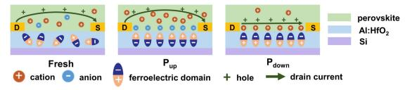
Fig. 4 The modulation mechanism of ferroelectric-gating for charge redistribution and ion mitigation in the perovskite phototransistor.
