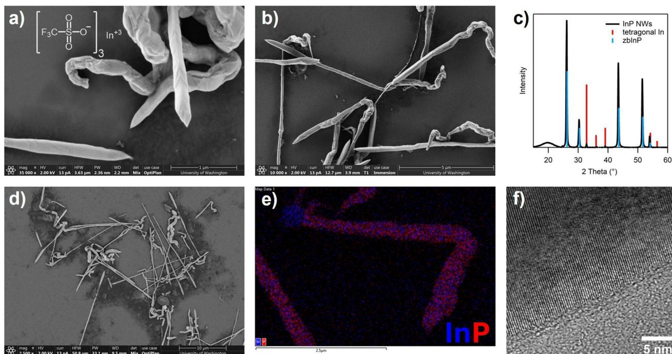
Fig. 4 Characterization of InP nanowires synthesized using  $\text{In}(\text{OTf})_3$  including SEM images (a, b and d), (c) PXRD pattern showing bulk zinc blende InP and a relatively low amount of tetragonal indium metal, (e) SEM-EDS map showing an InP nanowire growing out of an indium particle, and (f) high-resolution TEM image showing the (111) lattice planes of the edge of a nanowire.
