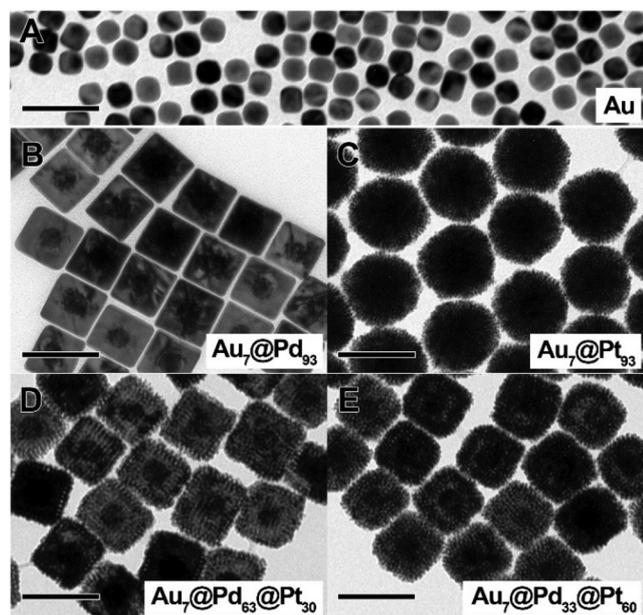
**Fig. 2** Synthesis of Au@Pt, Au@Pd and Au@Pd@Pt NCs. (A) Low-magnification TEM image of Au nanospheres used as seeds during the coating process. (B–E) TEM images of Au@Pd@Pt NCs with different compositions of metals: Au<sub>7</sub>@Pd<sub>93</sub> NCs (B), Au<sub>7</sub>@Pt<sub>93</sub> NCs (C), Au<sub>7</sub>@Pd<sub>63</sub>@Pt<sub>30</sub> NCs (D), and Au<sub>7</sub>@Pd<sub>33</sub>@Pt<sub>60</sub> NCs (E). Scale bars: 100 nm.
