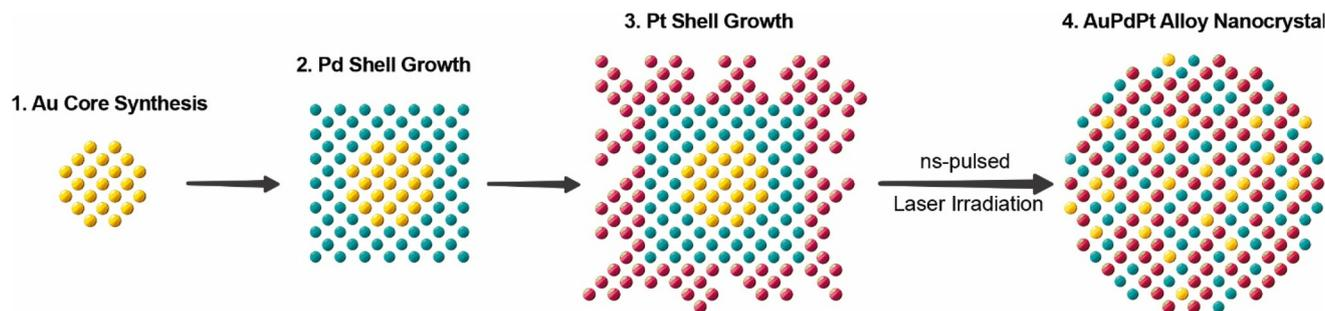
**Fig. 1** Schematic view of the synthesis of AuPdPt alloy NCs. After the synthesis of the Au core (1), Pd is first deposited to form a cubic Pd shell (2) followed by the reduction of Pt ions, leading to the growth of a dendritic Pt shell (3). The resulting core-shell-shell heterostructures are then rapidly heated with ns-pulsed laser irradiation to induce the formation of alloy NCs.
