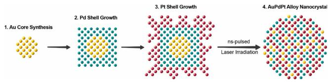
Fig. 1 Schematic view of the synthesis of AuPdPt alloy NCs. After the synthesis of the Au core (1), Pd is first deposited to form a cubic Pd shell (2) followed by the reduction of Pt ions, leading to the growth of a dendritic Pt shell (3). The resulting core-shell-shell heterostructures are then rapidly heated with ns-pulsed laser irradiation to induce the formation of alloy NCs.
