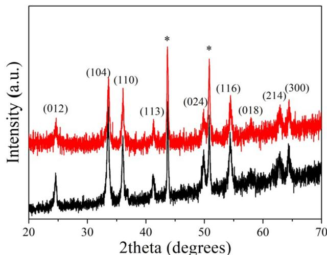
Fig. 1 XRD patterns of the bare  $\alpha\text{-Fe}_2\text{O}_3$  (black color) and the hybrid  $\alpha\text{-Fe}_2\text{O}_3/\text{Ox-Dex}$  electrodes.
