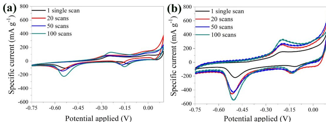
Fig. 5 CV curves of the bare  $\alpha\text{-Fe}_2\text{O}_3$  (a) and the hybrid  $\alpha\text{-Fe}_2\text{O}_3/\text{Ox-Dex}$  (b) electrodes in  $1 \text{ M}$   $\text{Li}_2\text{SO}_4$  solution recorded at 1, 20, 50, 100 scans.
