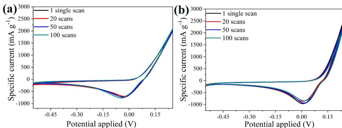
**Fig. 10** CV curves for 1, 20, 50, and 100 scans for the bare  $\alpha\text{-Fe}_2\text{O}_3$  (a) and the hybrid  $\alpha\text{-Fe}_2\text{O}_3/\text{Ox-Dex}$  (b) electrodes recorded in 1 M  $\text{Al}_2(\text{SO}_4)_3$  electrolyte solution.
