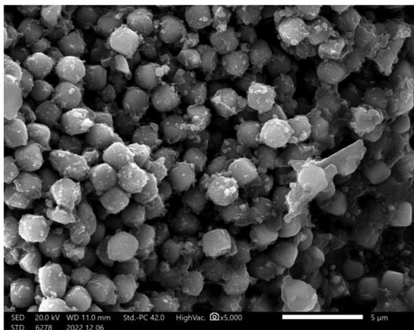
Fig. 8 FE-SEM image of the hybrid  $\alpha\text{-Fe}_2\text{O}_3/\text{Ox-Dex}$  electrode after 100 continuous intercalation/de-intercalation scans in 1 M  $\text{ZnSO}_4$  electrolyte solution.
