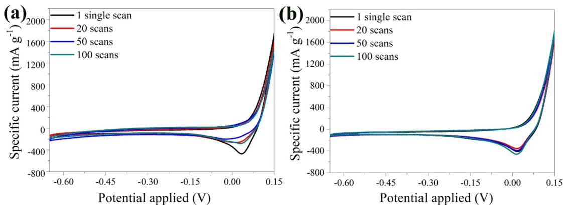
Fig. 7 CV curves of the bare  $\alpha\text{-Fe}_2\text{O}_3$  (a) and the hybrid  $\alpha\text{-Fe}_2\text{O}_3/\text{Ox-Dex}$  (b) electrodes in 1 M  $\text{ZnSO}_4$  electrolyte, recorded at 1, 20, 50, 100 scans.
