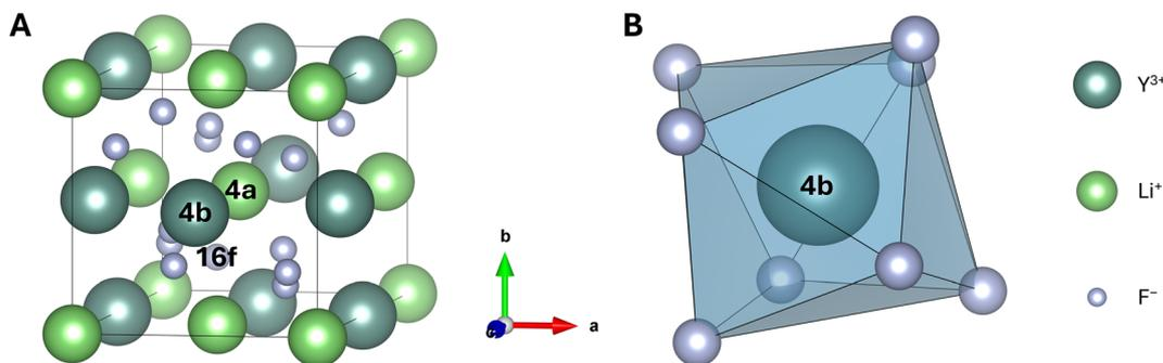
**Fig. 4** (A) Unit cell of LiYF<sub>4</sub> with the composition Li<sub>4</sub>Y<sub>4</sub>F<sub>16</sub>. Dark green spheres represent Y<sup>3+</sup>, light green spheres Li<sup>+</sup>, and small grey spheres represent F<sup>-</sup>. LiYF<sub>4</sub> features only one potential doping site, *i.e.*, Wyckoff position 4b. (B) Coordination polyhedron around Y<sup>3+</sup>. Each Y<sup>3+</sup> at a 4b site is surrounded by eight F<sup>-</sup> ions, creating a distorted square antiprism.
