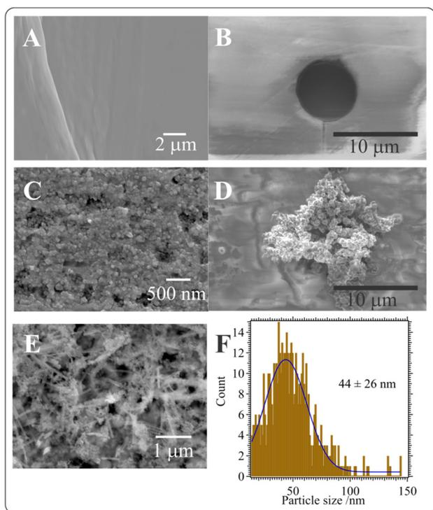
**Fig. 5** Scanning electron microscopy (SEM) micrographs of the initial polycrystalline Cu substrate (A) and after oxidation in pH 10 KHCO<sub>3</sub> (C) or pH 13 KOH (E). SEM images of the UME tip before (B) and after (D) the SECM tip distance experiments detailed in Fig. 1. (F) Histogram of NP sizes sampled from C using ImageJ software. The blue curve is a Gaussian curve fitting generated using Igor Pro software (version 9.0.5).
