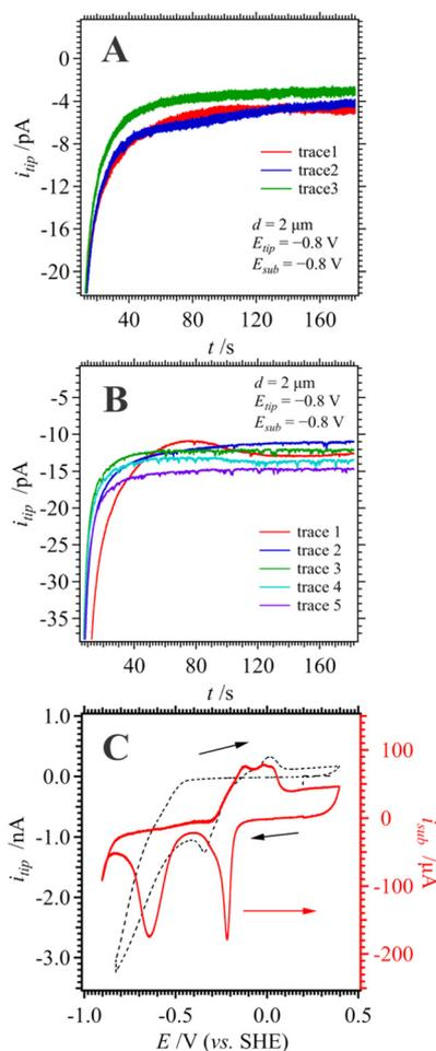
**Fig. 8** (A) Chronoamperograms recorded at  $i_{\text{tip}}$  while  $E_{\text{sub}}$  and  $E_{\text{tip}}$  were maintained at a cathodic potentials in a  $\text{KHCO}_3$  (pH 10) solution, and then (B) after performing the CVs depicted in (C) at  $0.020 \text{ V s}^{-1}$ . Red arrow indicates the current axis plotted against.
