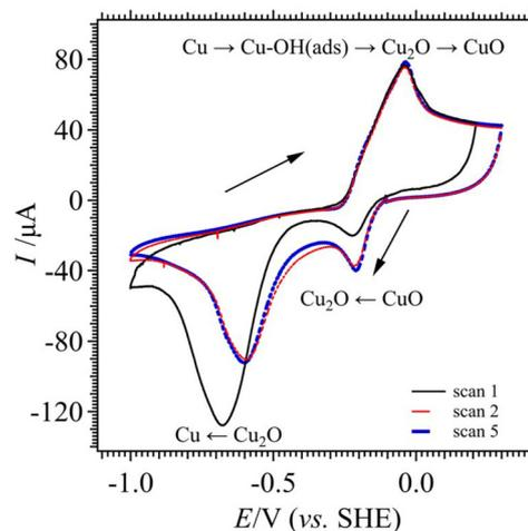
Fig. 2 Cyclic voltammograms (CVs) recorded using a polycrystalline Cu ( $\text{Cu}(\text{poly})$ ) substrate with a surface area of  $1 \text{ cm}^2$ , in a  $\text{KHCO}_3$  solution adjusted to pH 10 ( $\sim 0.5 \text{ M KHCO}_3$ ), at a scan rate of  $0.020 \text{ V s}^{-1}$ . The proposed surface reactions for each anodic and cathodic peak signal have been added in the inset. Multiple consecutive scans were performed as indicated in the inset.
