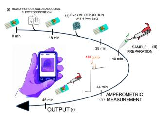
Fig. 1 Schematic representation of the preparation/sensing time: (i) highly porous gold nanocoral electrodeposition (hPGNC), (ii) alkaline phosphatase (AIP) immobilization with UV-Vis at  $\lambda$  = 405 nm in the presence of N-methyl-4(4'-formylstyryl)pyridinium (PVA-SbQ) as a photocrosslinked polymer, (iii) sample preparation encompassing the addition of ascorbate 2-phosphate (A2P) as an initial substrate, (iv) amperometric measurement of enzyme inhibition, and (v) final output.
