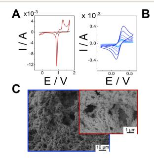
Fig. 2 (A) CVs of the bare gold screen printed electrode (black) and the hPGNC modified electrode (red) in 0.5 M H<sub>2</sub>SO<sub>4</sub>. Scan rate: 100 mV s<sup>-1</sup>. (B) CVs of the hPGNC modified electrode in 5 mM  $[Fe(CN)_6]^{3-/4-}$  in 10 mM HEPES buffer pH 7 (containing 100 mM Na<sub>2</sub>SO<sub>4</sub> as a supporting electrolyte) at increasing scan rates (colour coded) in the range 5-300 mV s<sup>-1</sup>. (C) SEM images of the hPGNC modified electrode.
