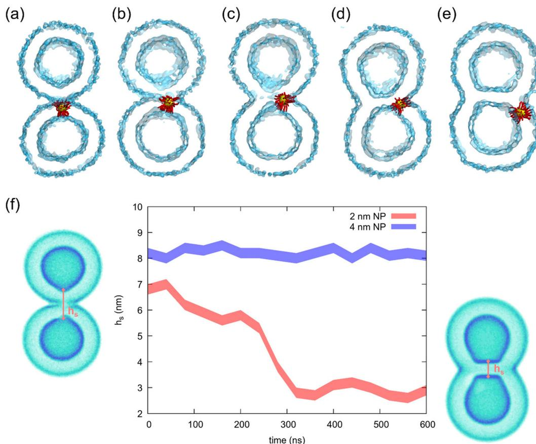
**Fig. 5** The molecular path from small AuNP-induced stalk to hemifusion, obtained from unbiased molecular dynamics simulations at 310 K. (a–e) Simulation snapshots that represent the different stages of the process. (f) The hydrophobic stalk height  $h_s$  as a function of time obtained from the unbiased simulations of the free vesicles with the two different NP core sizes. The stalk thinning leading to hemifusion is observed only in the case of the smaller core.
