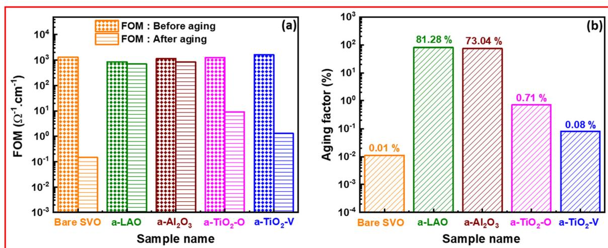
Fig. 5 (a) Figure of merit based on the  $\eta_T$  factor and the resistivity of the films. (b) The aging factor, denoted as the ratio between the FOM after aging and the FOM before aging. Both figures (a) and (b) are in logarithmic scale.
