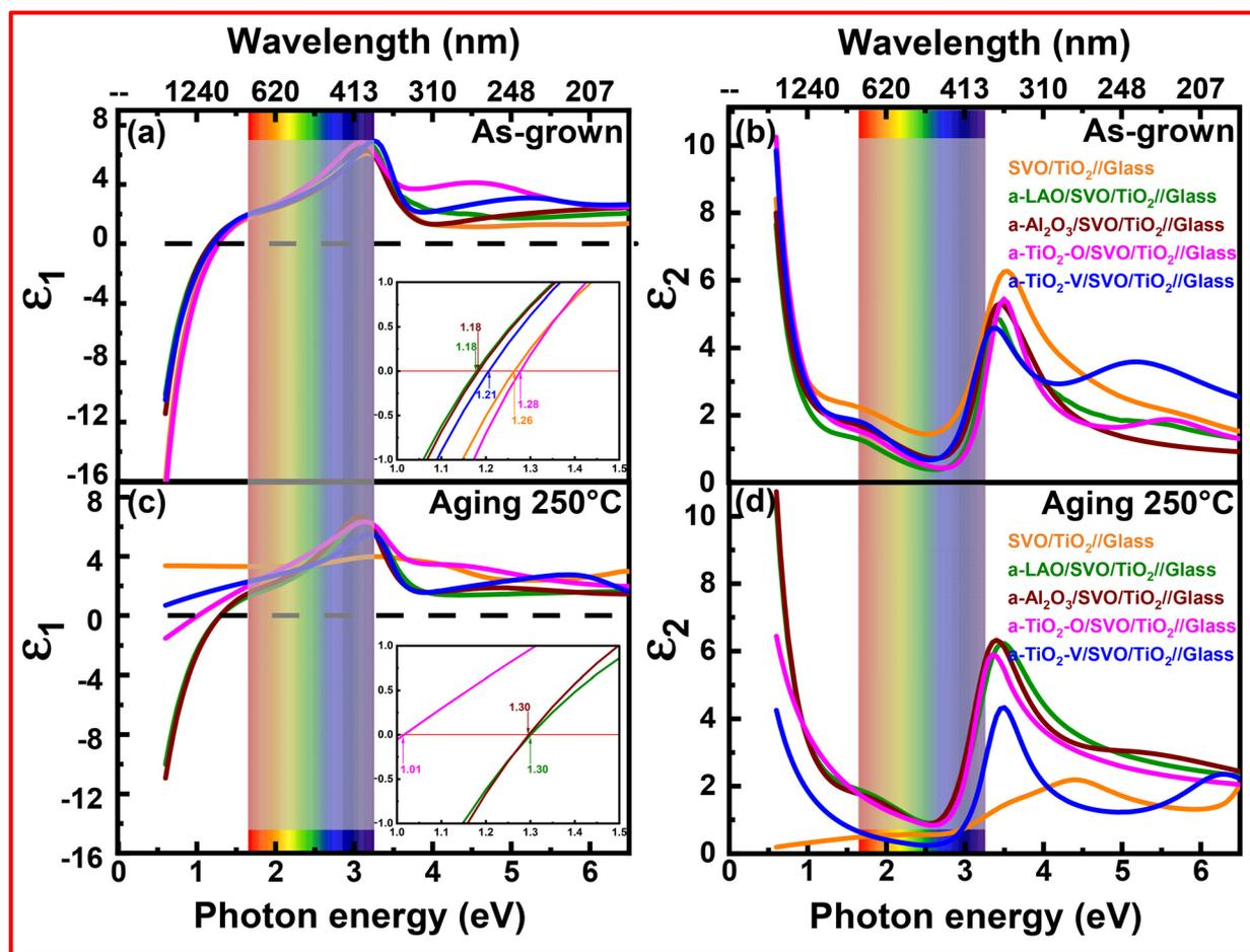
**Fig. 6** Spectroscopic ellipsometry measurements. (a and b) Real ( $\epsilon_1$ ) and imaginary ( $\epsilon_2$ ) parts of dielectric complex function ( $\epsilon = \epsilon_1 + i\epsilon_2$ ) of as grown polycrystalline SVO thin films with different capping layers. (c and d) Real and imaginary parts of SVO films with various capping layers' after annealing for 24 h in air. The inset in (a and c) is a zoom between 1 and 1.5 eV.
