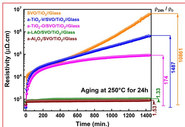
**Fig. 2** The variation of electrical resistivity of SVO thin films with and without capping layers, during heat treatment of the samples on a hot plate at 250 °C for 24 h in air atmosphere.
