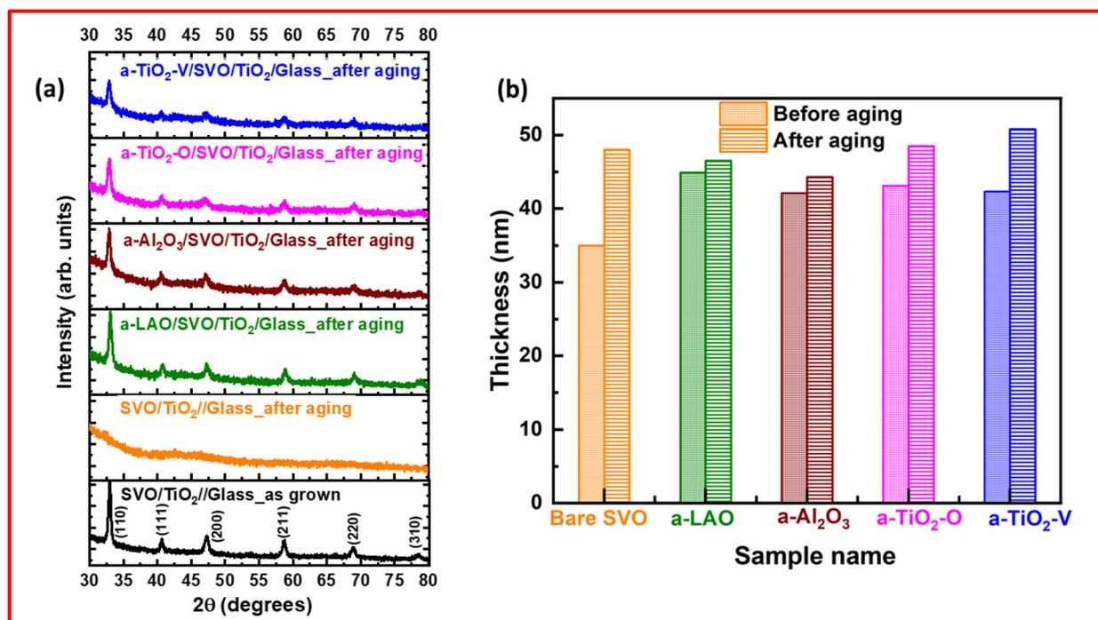
Fig. 1 (a) GIXRD patterns of SVO thin films grown on TiO<sub>2</sub> buffered glass substrate without and with different capping layers, after heat treatment at 250 °C for 24 h in air. (b) Effect of annealing temperature on the thickness of the samples before and after heat treatment.
