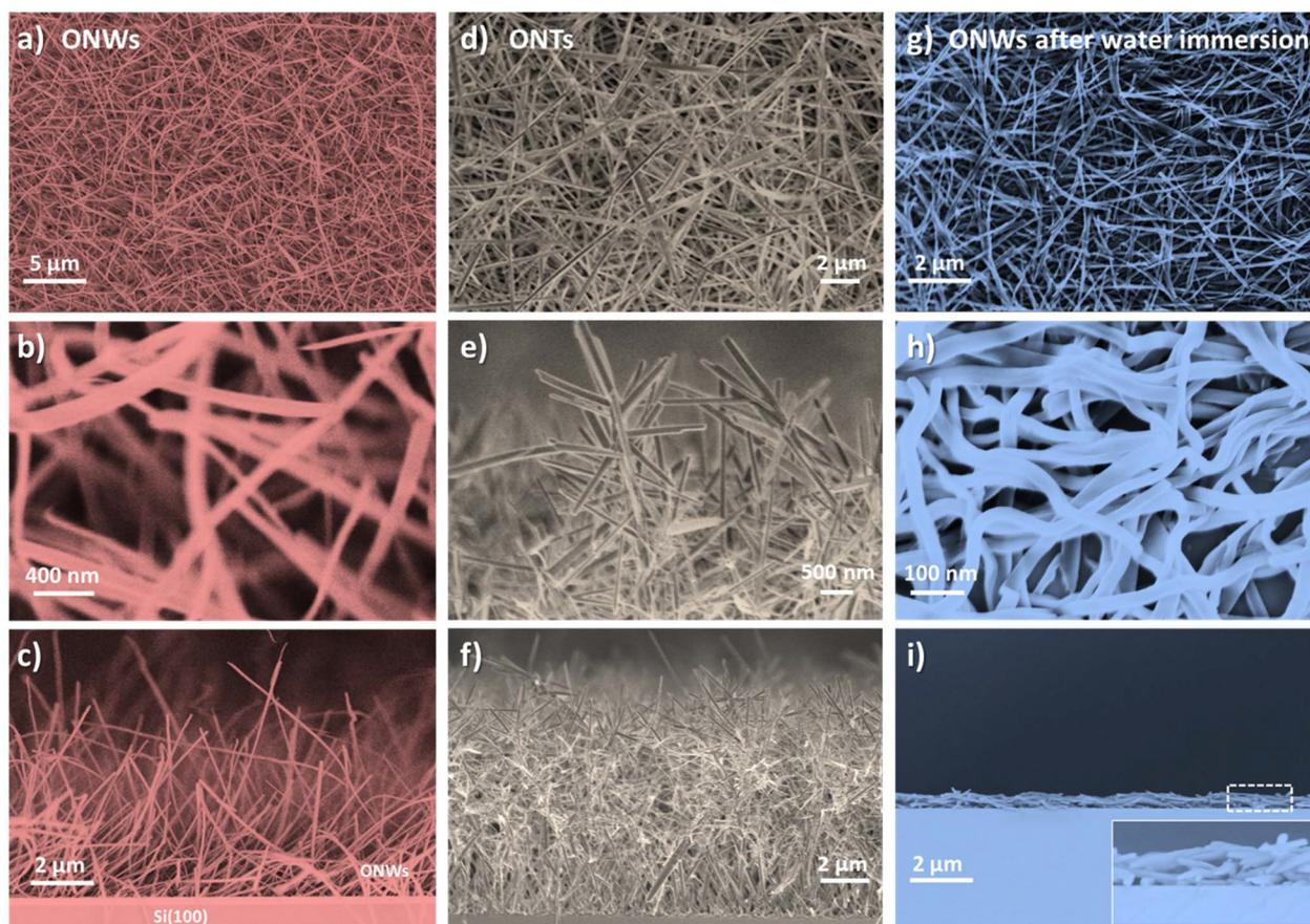
**Fig. 1** SEM micrographs of the H<sub>2</sub>Pc ONWs deposited on a silicon wafer decorated with gold nanoparticles with planar views in panels (a and b) and cross-section in panel (c). SEM micrographs in a planar view (d) and cross-section (e and f) of the H<sub>2</sub>Pc ONTs. (g–i) Characteristic SEM micrographs of the supported ONWs after immersion in distilled water.
