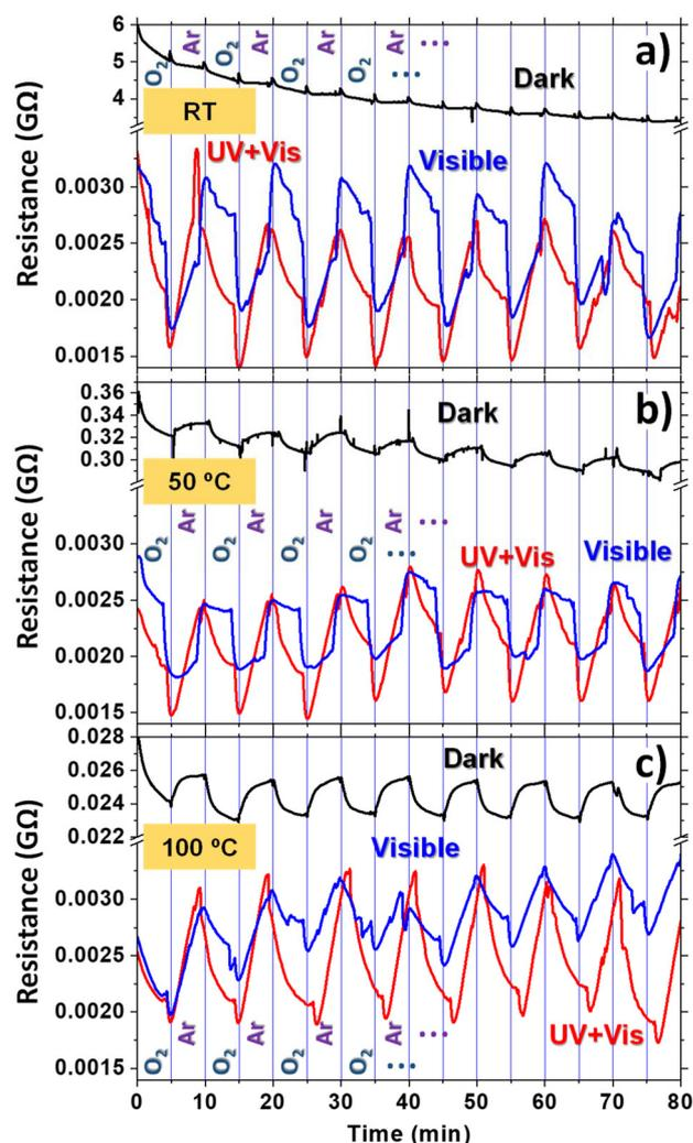
**Fig. 5** Organic nanotree sensor response to oxygen and argon at RT (a), 50 °C (b), and 100 °C (c) without irradiation (black line), under visible light irradiation (blue), and under UV + visible light irradiation (red).
