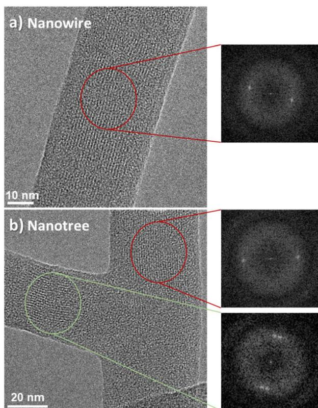
**Fig. 2** High-resolution transmission electron micrographs corresponding to an H<sub>2</sub>Pc nanowire (a) and the connected primary and secondary wires in an H<sub>2</sub>Pc nanotree (b). Digital diffraction patterns (DDPs) of the selected areas (right side of the figure) revealing the crystalline character of the ONWs and ONTs.
