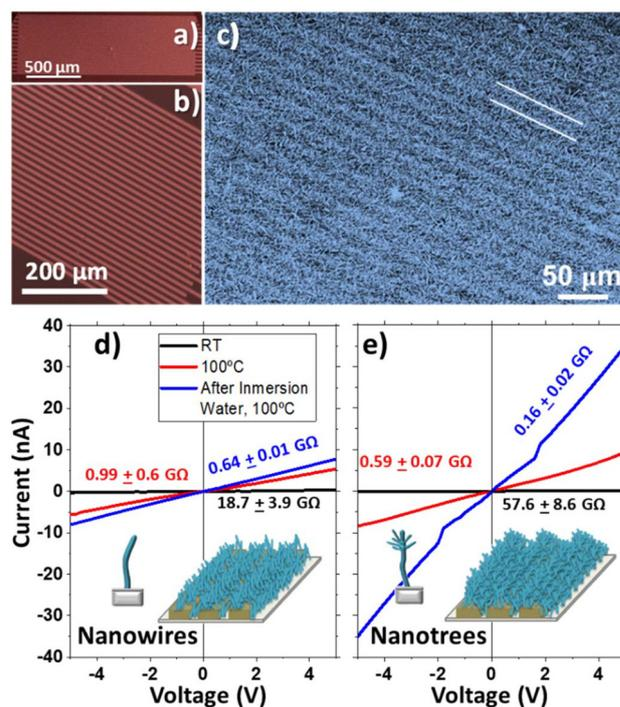
**Fig. 3** SEM images of the commercial interdigitated electrodes before (a and b) and after (c) the deposition of H<sub>2</sub>Pc nanotrees. *I*–*V* curves for the ONWs (d) and ONTs (e) on commercial electrodes at room temperature (black) and 100 °C (red) under a constant argon flux at ambient pressure. In addition, the *I*–*V* response of the device is shown after the water immersion treatment and subsequent drying. These curves were recorded at 100 °C under an Ar flux (blue curves).
