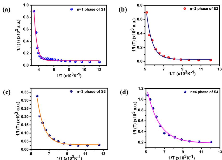
Fig. 3 Inverse of integrated PL intensity  $[1/I(T)]$  vs. inverse of temperature ( $1/T$ ) plots fitted (solid lines) using eqn (1) for (a) S1, (b) S2, (c) S3 and (d) S4.
