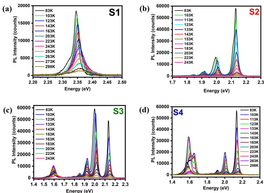
Fig. 2 Temperature-dependent PL spectra of the  $(\text{TEA})_2(\text{MA})_{n-1}\text{Pb}_n\text{I}_{3n+1}$  thin films at different temperatures from 83 to 298 K. Panels (a–d) correspond to samples S1–S4, respectively. The excitation wavelengths were 405 nm for S1 and 532 nm for S2–S4.
