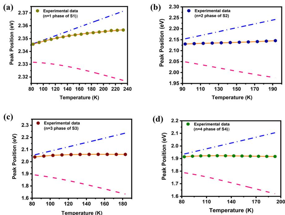
Fig. 5 (a–d) Temperature-dependent PL peak positions of the main phases of samples S1–S4, respectively, fitted with eqn (3) (solid lines). The dashed-dotted (blue) and dashed (pink) lines show the individual contributions of thermal expansion and exciton–phonon interaction, respectively.
