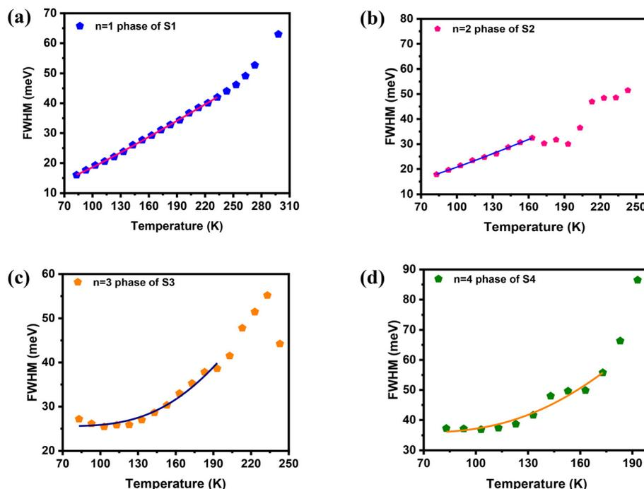
Fig. 7 (a–d) Temperature-dependent full width at half maximum (FWHM) of the main PL peaks of the  $(\text{TEA})_2(\text{MA})_{n-1}\text{Pb}_n\text{I}_{3n+1}$ ,  $n = 1-4$  films. The solid lines represent the fitting results using eqn (8).
