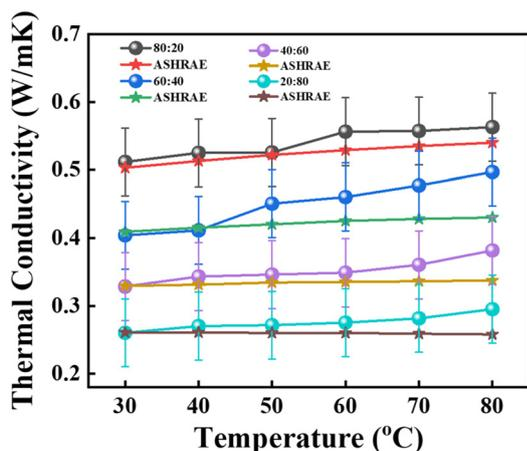
**Fig. 8** TC of DI water and PG mixture with different volumes and compared with ASHRAE data.<sup>28</sup>
