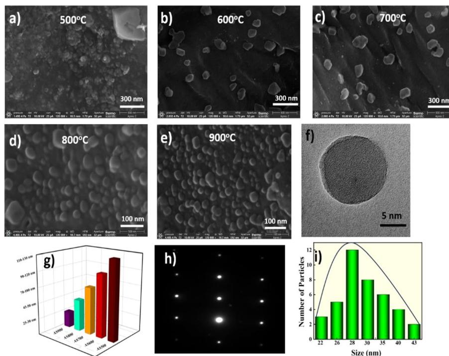
**Fig. 2** (a–e) FESEM images at temperatures ranging from 500 to 900 °C, respectively. (f) TEM image of AS900, (g) the particle sizes of different nanoparticles, (h) SAED pattern of AS900, (i) histogram of AS900.
