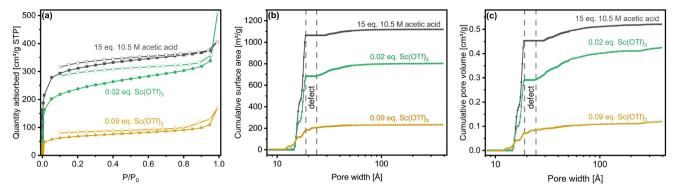
Fig. 7 Representative (a)  $N_2$  adsorption and desorption isotherms (77K), (b) cumulative surface areas, and (c) cumulative pore volumes of activated COF-LZU1 synthesized under different catalytic conditions.
