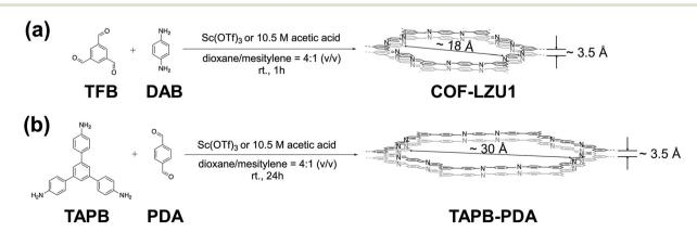
Scheme 1 Synthesis routes to (a) COF-LZU1 and (b) TAPB-PDA using either acetic acid or Sc(OTf)<sub>3</sub> as catalyst.
