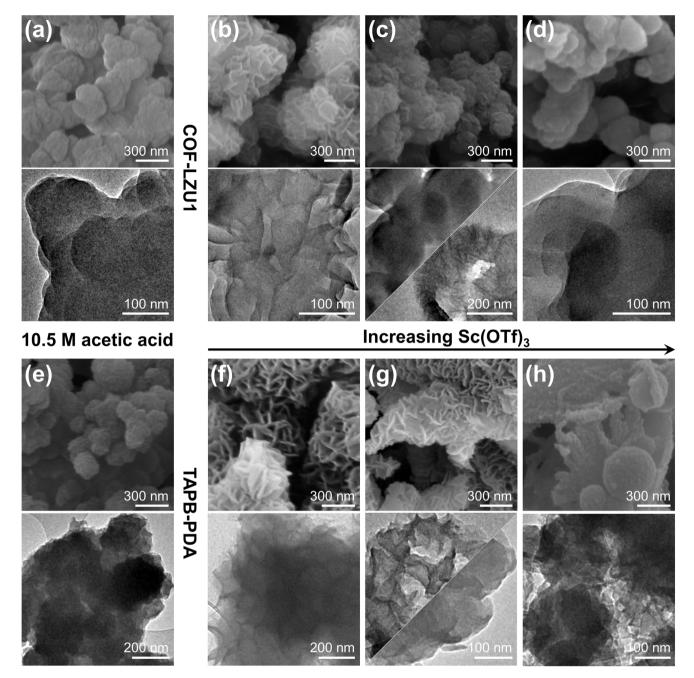
Fig. 1 SEM and TEM images of COF-LZU1 synthesized under (a) 15 eq. 10.5 M acetic acid and (b) 0.02, (c) 0.04, and (d) 0.09 eq. Sc(OTf)<sub>3</sub>; and TAPB-PDA synthesized under (e) 20 eq. 10.5 M acetic acid and (f) 0.02, (g) 0.09, and (h) 0.15 eq. Sc(OTf)<sub>3</sub>.
