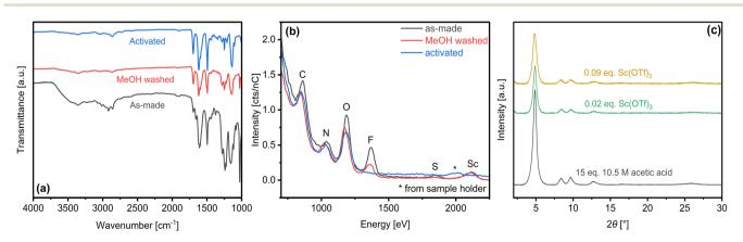
Fig. 6 (a) FTIR spectra and (b) average LEIS spectra over 3nm sputtering depth for 0.09 eq. Sc(OTf)<sub>3</sub>-derived COF-LZU1 at points along the solvent activation process. (c) PXRD patterns of activated COF-LZU1 synthesized under different catalytic conditions.
