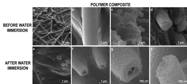
**Fig. 6** SEM imaging of the two-side sputtered mat coated with polyamide: top-view (a and b) and cross-section (c and d). SEM imaging of the cross-section of the two-side sputtered mat coated with polyamide after water immersion at different magnifications (e–h).
