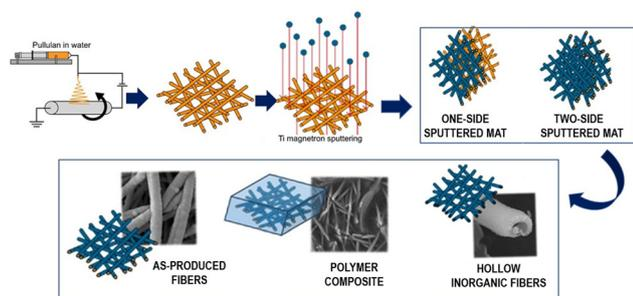
**Fig. 1** Schematic representation of pullulan electrospinning and Ti magnetron sputtering on the nanofibers for obtaining one-side and two-side sputtered mats. The as-produced fibers were embedded in a thermoplastic matrix for the development of polymer composites and also exploited for the development of hollow inorganic fibers.
