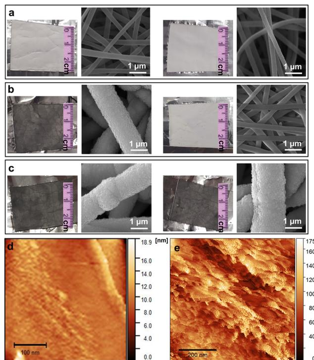
**Fig. 2** Macroscopic views and SEM-FEG imaging of the two mat faces (upper one on the left and lower one on the right) of the as-spun mat (a), one-side sputtered mat (b), and two-side sputtered mat (c). AFM characterization of the as-spun mat (scale bar 100 nm) (d) and the Ti-sputtered face of the one-side sputtered mat (scale bar 200 nm) (e).
