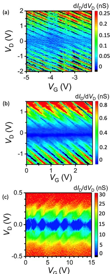
**Fig. 4** 2D  $dI_D/dV_D$  mapping of PbS QD transistors. Contour mapping stability diagrams were obtained by plotting colour maps of  $dI_D/dV_D$  as functions of  $V_D$  and  $V_G$  for (a) 1,4-Butanedithiol (BuDT)-anchored PbS QD RTT, (b) 1,2-ethanedithiol (EDT)-anchored PbS QD RTT, and (c) oleic acid-capped PbS QD SET. All measurements were carried out at  $T = 9$  K.
