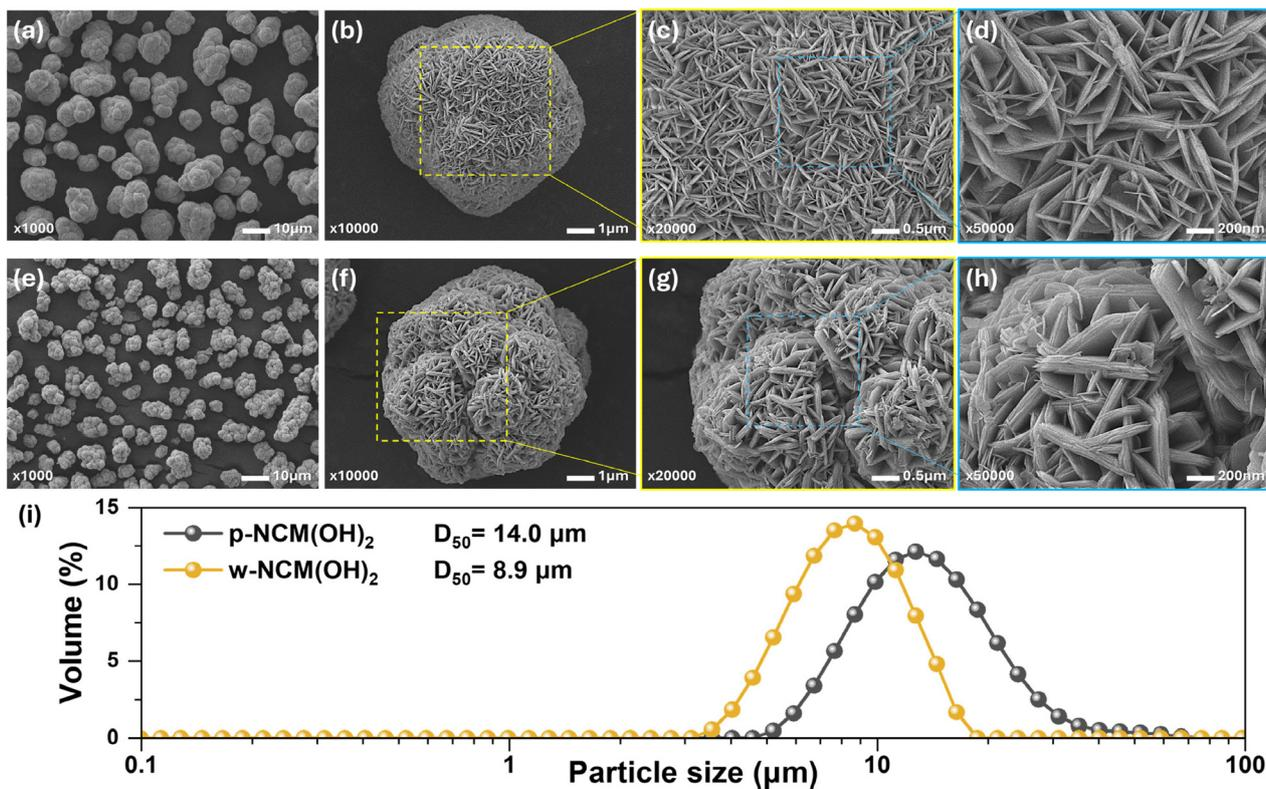
Fig. 1 SEM images of (a–d) p-NCM(OH)<sub>2</sub> and (e–h) w-NCM(OH)<sub>2</sub> precursors at various magnifications, along with the corresponding (i) particle size distribution analysis.
