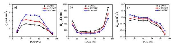
Fig. 11 The calculated kinetic parameters (a) exchange current density, (b) charge transfer resistance, and (c) Li<sup>+</sup> diffusion coefficient of the CAMs.
