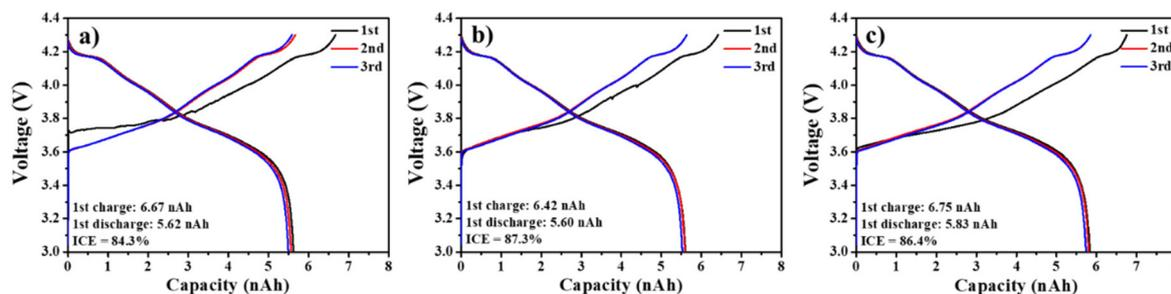
Fig. 9 Galvanostatic charge–discharge voltage profiles of (a) p-LNCM, (b) w-LNCMW, and (c) s-LNCMW cathode materials measured at 2 nA using a microcavity electrode.
