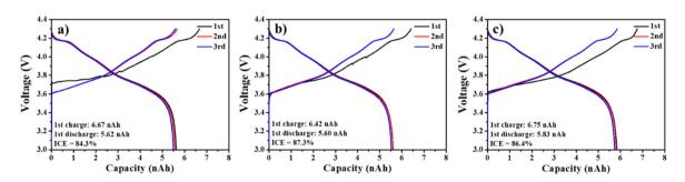
Fig. 9 Galvanostatic charge-discharge voltage profiles of (a) p-LNCM, (b) w-LNCMW, and (c) s-LNCMW cathode materials measured at 2 nA using a microcavity electrode.
