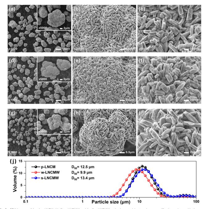
Fig. 2 SEM images of (a-c) p-LNCM, (d-f) w-LNCMW and (g-i) s-LNCMW cathode materials at various magnifications, along with the corresponding (j) particle size distribution analysis.
