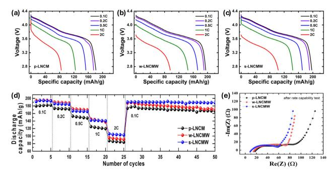
Fig. 8 Galvanostatic discharge voltage curves of (a) p-LNCM, (b) w-LNCMW and (c) s-LNCMW cathode materials at specified current densities. (d) Rate capability performance of CAMs at 0.1C, 0.2C, 0.5C, 1C and 2C for 5 cycles. (e) PEIS results presented as Nyquist plots for CAMs after rate capability test.
