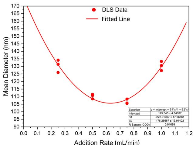
**Fig. 3** Collected data for particle size measured using DLS for four ethanol addition rates:  $0.25$ ,  $0.5$ ,  $0.75$ , and  $1.0 \text{ mL min}^{-1}$  (each with  $n = 3$ ). A quadratic regression was performed on the data, with the line of best fit indicating a local minimum in particle size associated with an addition rate of  $0.629 \text{ mL min}^{-1}$ , which was rounded down to  $0.625 \text{ mL min}^{-1}$  for purposes of simplifying calculations.
