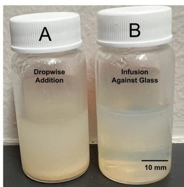
**Fig. 2** Nanoparticle samples synthesized using (A) dropwise ethanol addition and (B) infusion against the glass, both at a rate of  $1 \text{ mL min}^{-1}$ . Photo taken when both samples were about 10 months old. Dropwise addition is a source of inhomogeneity in the reaction mixture, with subsequent syntheses having varying degrees of sedimentation that are significantly higher than syntheses using infusion against the glass.
