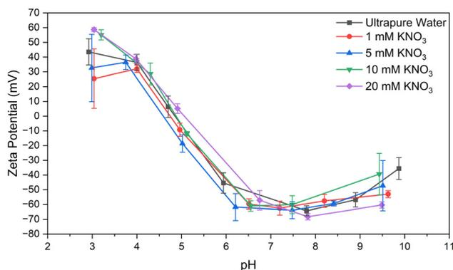
**Fig. 6** Zeta potential of BSA nanoparticles synthesized in several different concentrations of KNO<sub>3</sub>, all washed and redispersed in 1 mM KNO<sub>3</sub> ( $n = 3$  for each electrolytic strength). Regardless of electrolytic strength during synthesis, zeta potential of the washed dispersion was effectively unchanged, and the isoelectric point remained similar to that of naked albumin.
