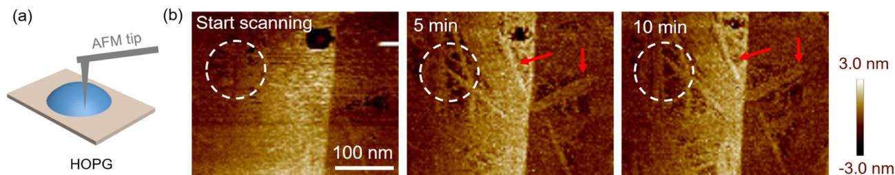
**Fig. 4** *In situ* capture of the growth of peptide/FG filaments on the HOPG surface. (a) Schematic diagram of the AFM tip deposited in solution. The temperature was 24 °C and the humidity was 60%. (b) Captured AFM images at the start, 5 min and 10 min, respectively. The dashed line circle and arrays show the dynamic formation of filaments.
