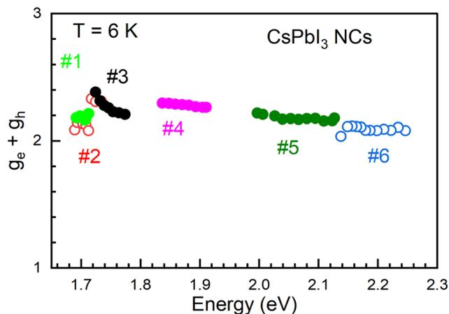
Fig. 5 Spectral dependence of the bright exciton  $g$ -factor in CsPbI<sub>3</sub> NCs, calculated from the electron and hole  $g$ -factors as  $g_{\text{BX}} = g_e + g_h$ . For the samples #1 to #4, the experimental values for  $g_e$  and  $g_h$  are taken. For the samples #5 and #6, we take the experimental values of  $g_h$  and the modeled values of  $g_e$  from ref. 14.
