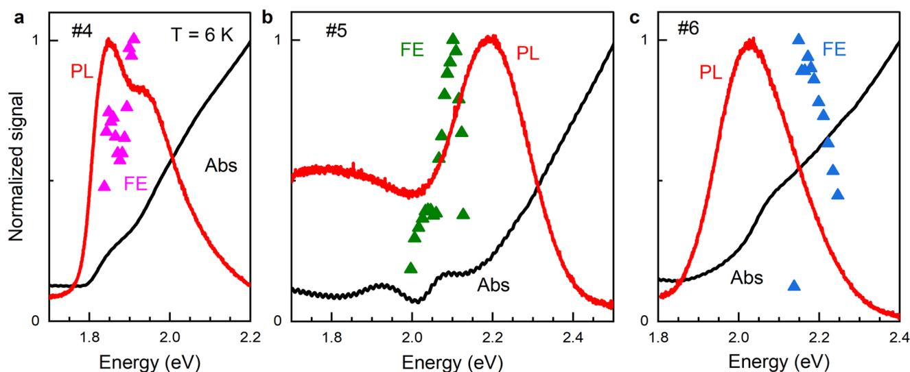
**Fig. 1** Spectral dependences of the photoluminescence intensity (red line), absorption (black line), and Faraday ellipticity amplitude (symbols) in CsPbI<sub>3</sub> NCs (samples #4, #5, and #6), measured at the temperature of 6 K.
