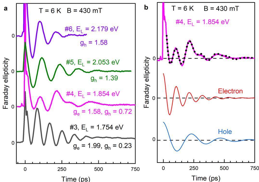
**Fig. 2** (a) Spin dynamics in the CsPbI<sub>3</sub> NCs (samples #3, #4, #5 and #6) in 430 mT magnetic field. (b) The upper graph shows the FE dynamics in sample #4. Black dotted line is a fit with eqn (2). The two lower graphs show the oscillatory components in the spin dynamics, corresponding to the electron (red line,  $|g_e| = 1.58$  and  $T_{2,e}^* = 150$  ps) and the hole (blue line,  $|g_h| = 0.72$  and  $T_{2,h}^* = 220$  ps).
