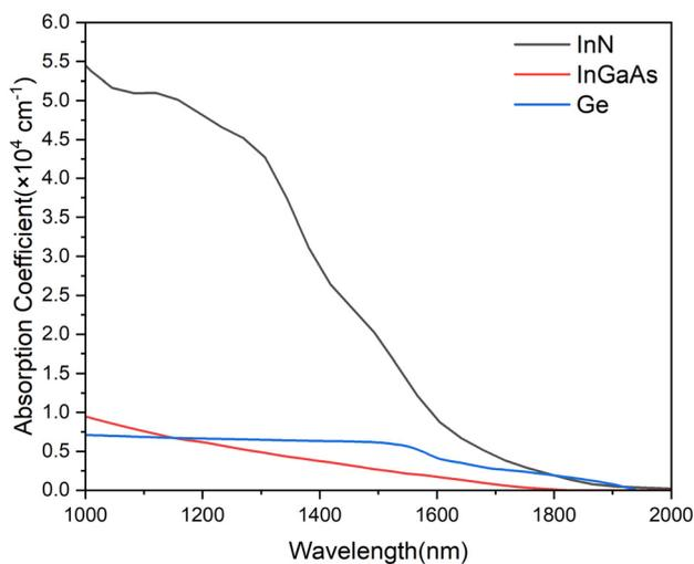
**Fig. 1** Comparison of the absorption coefficients of InN, InGaAs,<sup>3</sup> and Ge<sup>4</sup> with the responsivity performance of detectors with the same device structure in the SWIR range.
