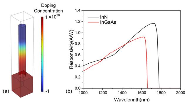
**Fig. 8** (a) The doping configuration of the repeating NW unit in periodic arrays. Red represents n-type doping and blue represents p-type doping. (b) The responsivity curve of InN and the InGaAs NW array within the SWIR range.
