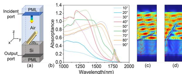
**Fig. 7** (a) The periodic model of the inclined InN NW array. (b) The absorption spectrum of the NW array is dependent on the inclination angle  $\alpha_3$  under TE-polarized light. The cross-section of distribution of the electric field intensity  $|E|$  inside the inclined InN NW under TE-polarized incidence at  $\lambda = 1300$  nm: (c)  $\alpha_3 = 20^\circ$  and (d)  $\alpha_3 = 50^\circ$ .
