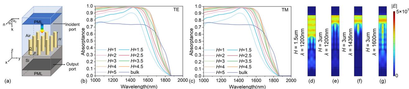
**Fig. 4** (a) The periodic model of the InN NW array. The absorption spectrum of NW arrays under (b) TE- and (c) TM-polarized incidence. (d)–(g) The longitudinal section of distribution of the electric field intensity  $|E|$  inside the 3D hexagonal InN NW under TE-polarized incidence with different NW heights and incident wavelengths.
