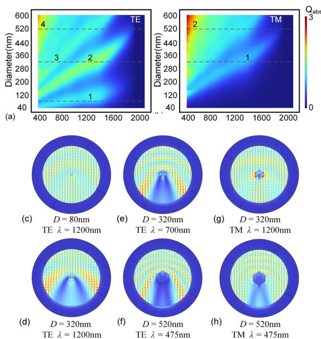
**Fig. 3**  $Q_{\text{abs}}$  of the single hexagonal InN NW as a function of  $\lambda$  and  $D$  under (a) TE- and (b) TM-polarized illumination. Distribution of the electric field intensity  $|E|$  inside the hexagonal InN NW for the corresponding peak indicated by grey dashed lines: (c)–(f) the 1st enhanced peak to the 4th enhanced peak under TE-polarized incidence; (g) and (h) the 1st enhanced peak to the 2nd enhanced peak under TM-polarized incidence.
