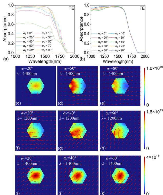
**Fig. 6** (a) Absorptance as a function of wavelength and elevation angle  $\alpha_1$ . (b) Absorptance as a function of wavelength and azimuth angle  $\alpha_2$  when  $\alpha_1$  is set to  $40^\circ$ . (c)–(e) The optical power loss spectrum and the Poynting vector of different angles  $\alpha_1$  at 1400 nm. (f)–(k) The optical power loss spectrum and the Poynting vector of different angles  $\alpha_2$  at 1200 nm and 1400 nm.
