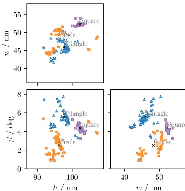
Fig. 5 Dimensional reconstruction solutions of the  $\text{Si}_3\text{N}_4$  nanograting from Fig. 1, obtained by minimizing the weighted  $\chi_\gamma^2$ -function in eqn (6) for various weighting parameters between  $\gamma = 0$  (fluorescence only) and  $\gamma = 1$  (scattering only). The solutions are grouped into clusters labeled with different markers and colors.
