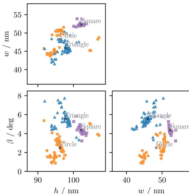
Fig. 5 Dimensional reconstruction solutions of the  $\text{Si}_3\text{N}_4$  nanograting from Fig. 1, obtained by minimizing the weighted  $\chi^2$ -function in eqn (6) for various weighting parameters between  $\gamma = 0$  (fluorescence only) and  $\gamma = 1$  (scattering only). The solutions are grouped into clusters labeled with different markers and colors.
