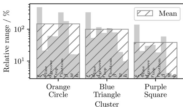
**Fig. 6** Comparison of the relative ranges for  $\text{Si}_3\text{N}_4$  nanograting parameters from Table 1, plotted across different solution clusters as shown in Fig. 5. The comparison shows that Cluster Purple Square has the smallest relative parameter ranges, while Cluster Orange Circle has the largest.
