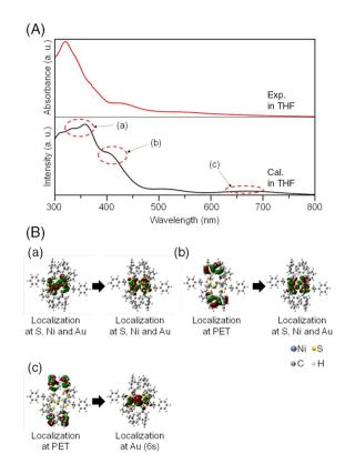
Fig. 4 (A) Experimental (red) and calculated (black) absorption spectra of  $[AuNi_6(PET)_{12}]^+$  in THF. (B) (a)–(c) Molecular orbitals of  $[AuNi_6(PET)_{12}]^+$  for the main peaks observed in the calculated spectrum in THF in (a)–(c) of (A).
