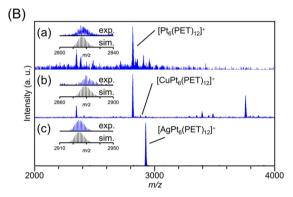
Fig. 5 Positive-ion MALDI-mass spectra (a) before and after adding (b) Cu(i) and (c) Ag(i) salts into (A)  $Pd_6(PET)_{12}$  and (B)  $Pt_6(PET)_{12}$  solutions. The insets show the comparison of the isotope patterns between the experimental spectrum (blue) and the calculated one (black). Several peaks attributed to byproducts are assigned and summarized in Tables S5 and S6.†
