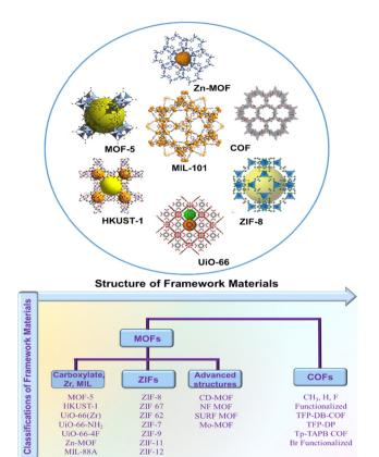
Fig. 1 Structure of various framework materials and their classifications.
