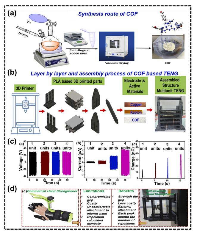
Fig. 8 (a) Synthesis route of COF; (b) layer-by-layer and assembly process of COF-based TENG; and (c) multi-unit TENG voltage, current, charge output of the 4 units of COF-based TENG connected in parallel connection, (d) comparison between commercial system and self-powered hand strengthening device. Reprinted from ref. 17, Copyright © 2022, Elsevier.
