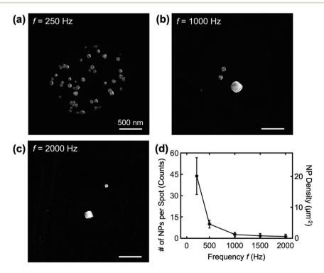
Fig. 4 Frequency vs. number of Pt nanoparticles. (a–c) SEM images of nanocubes deposited at different f (a) 250, (b) 1000, and (c) 2000 Hz. (d) Number of nanoparticles per spot (left) and nanoparticle density (right) vs frequency of the square wave. Deposition conditions:  $E_U = 1.24 \text{ V}$ ,  $E_L = -0.275 \text{ V}$ , and  $t_d = 5 \text{ s}$ .
