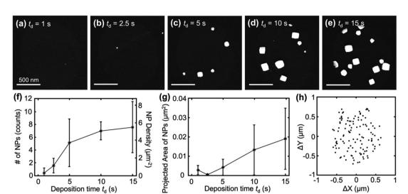
Fig. 5 Size control of Pt nanocubes (a–e) SEM images of nanocubes electrodeposited with varying the deposition time  $t_d$  from 1 to 15 s ( $E_U = 1.24$  V,  $E_L = -0.275$  V, and f = 500 Hz) (f and g) Relationships between (f) the number of synthesized particles and (g) the projected area of the deposited particles at different  $t_d$  from 0 to 15 s. (h) Scatter plot showing particle offsets measured from total 120 Pt nanoparticles electrodeposited with varying  $t_d$ .
