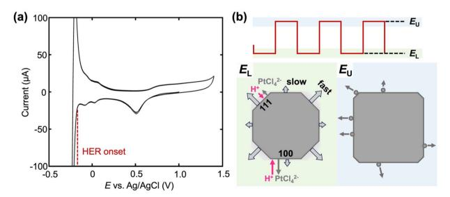
Fig. 6 Proposed mechanism of Pt nanoparticle growth. (a) Cyclic voltammogram showing the onset of HER on Pt disk electrode (2 mm diameter). Three consecutive cycles are shown with an initial potential of 1 V. Solution: 100 mM  $H_2SO_4$ ; reference electrode: Ag/AgCl; counter electrode: Pt wire; scan rate: 0.1 V s<sup>-1</sup>. (b) Schematic illustration of square-wave potential waveform oscillating between upper ( $E_U$ ) and lower ( $E_L$ ) potentials.
