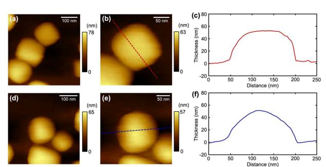
Fig. 2 AFM of the electrosynthesized Pt nanoparticles. (a and b) Topographic AFM images of cubic Pt nanoparticles and (c) the line profile. Deposition conditions:  $E_L = -0.275 \text{ V}$ ,  $E_U = 1.24 \text{ V}$ , f = 500 Hz, and  $t_d = 5 \text{ s}$ . (d and e) Topographic images of rounded Pt nanoparticles and (f) the line profile. Deposition conditions:  $E_L = -0.1 \text{ V}$ , rest conditions are the same as (a)–(c).
