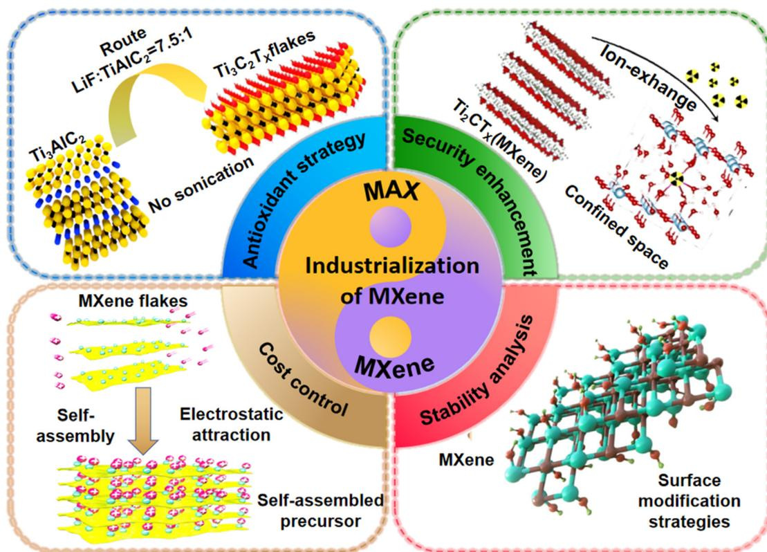
**Fig. 1** Optimization strategy of MXene scale preparation. Figure used in the top left corner: reproduced from ref. 14 with permission from Wiley-VCH, copyright 2016. Figure used in the top right corner: reproduced from ref. 15 with permission from Elsevier, copyright 2019. Figure used in the lower left corner: reproduced from ref. 20 with permission from Wiley-VCH, copyright 2018. Figure used in the lower right corner: reproduced from ref. 24 with permission from Elsevier, copyright 2023.
