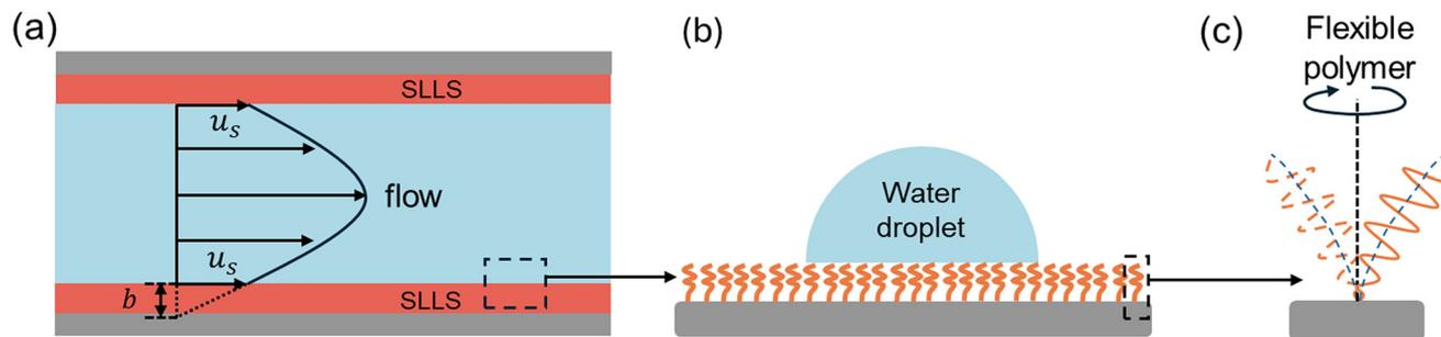
**Fig. 1** (a) The schematic of a microchannel with slippery liquid-like surfaces (SLLSs) as the channel surfaces. When liquid is running through the microchannel, a fluid slip will be induced at the liquid–SLLS interface. The  $u_s$  is the fluid slip velocity at the liquid–SLLS interface, and  $b$  is the slip length which is the extended length to which the fluid velocity vanishes. (b) Zoom-in image of the SLLS made by grafting (c) flexible polymers to a substrate.
