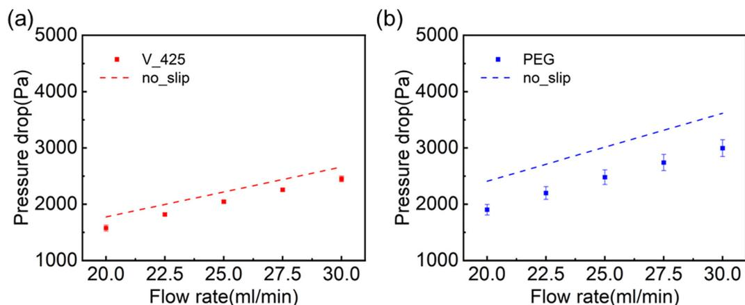
**Fig. 4** Shows the pressure drop measurements for both (a) hydrophobic (V\_425) and (b) hydrophilic (PEG) slippery liquid-like surfaces at different flow rates. The dots represent the experimental results, while the dashed lines represent the theoretical pressure values at the no-slip boundary condition.
