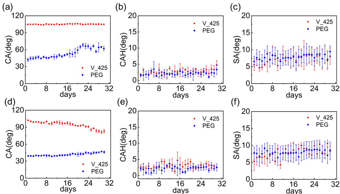
**Fig. 6** (a)–(c) Change in the wetting properties *i.e.*, CA, CAH, and SA, of slippery liquid-like surfaces with time while exposed in an air environment; (d)–(f) change in wetting properties, *i.e.*, CA, CAH, and SA, of the slippery liquid-like surface while being immersed in DI water.
