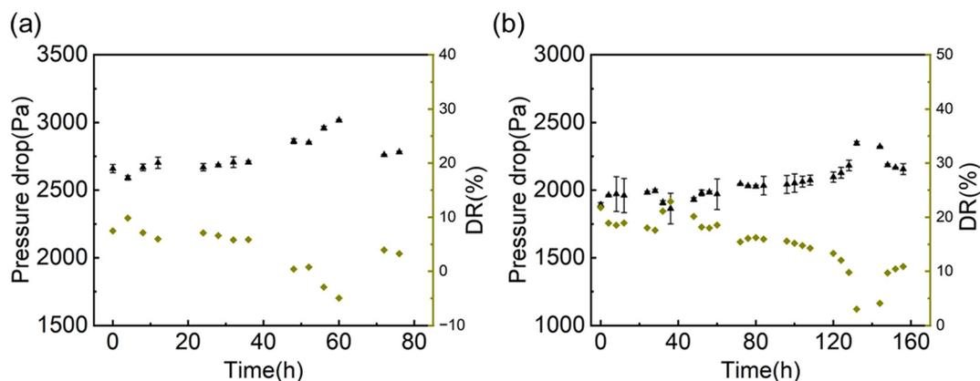
**Fig. 7** (a) Hydrodynamic durability test shows the change in the pressure drop (left axis) and drag reduction coefficient (right axis) over time for the hydrophobic slippery liquid-like surface. The drag reduction reduced below 0 at 56 h. (b) Hydrodynamic durability test shows the change in pressure drop (left axis) and drag reduction (right axis) over time for the hydrophilic slippery liquid-like surface. The drag reduction remained around 10% after 1 week.
