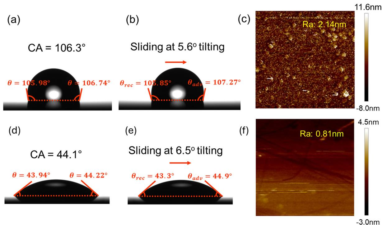
**Fig. 3** (a)–(c) present the single measurement of CA, CAH and SA values and the AFM roughness measurement on a  $3 \mu\text{m} \times 3 \mu\text{m}$  area for the hydrophobic slippery liquid-like surface. (d)–(f) show the single measurement of CA, CAH and SA values and the AFM roughness measurement using a  $3 \mu\text{m} \times 3 \mu\text{m}$  area for the hydrophilic slippery liquid-like surface.
