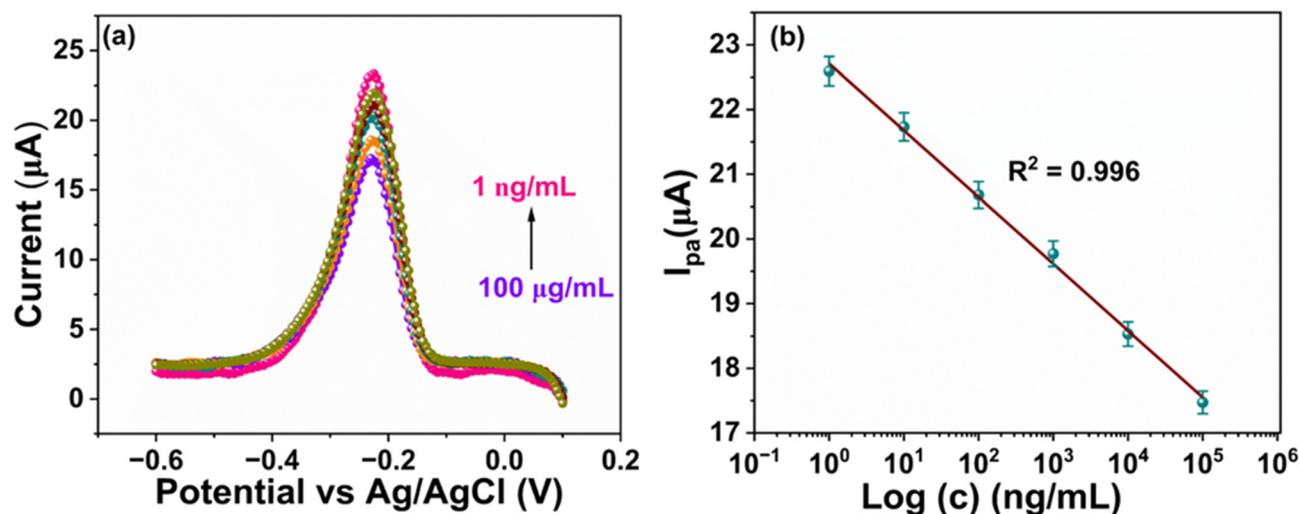
Fig. 5 (a) Square wave voltammetric profiles at various concentrations of the recombinant HER-2 protein ranging from 1 ng mL<sup>-1</sup> to 100 µg mL<sup>-1</sup>. (b) Sensor calibration graph was achieved at 0.22 V (–220 mV), showing a linear correlation between the peak current ( $I_{pa}$ ) and the HER-2 recombinant protein concentrations.
