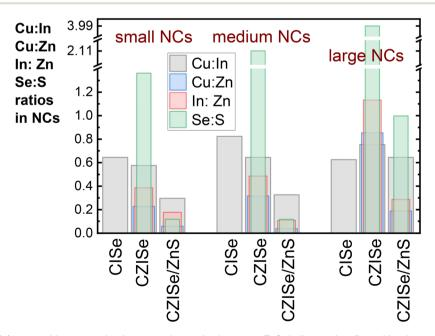
Fig. 4 Changes of the NCs' composition upon zinc incorporation and subsequent ZnS shell growth reflected by the corresponding element ratios: Cu: In, Cu: Zn, In: Zn, and Se: S.
