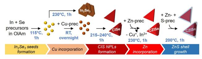
Fig. 1 Scheme of the synthesis of In<sub>2</sub>Se<sub>3</sub> nanosheets, triangular CISe NCs, CZISe, and core/shell CZISe/ZnS NCs.
