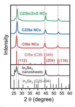
Fig. 2 XRD patterns of In<sub>2</sub>Se<sub>3</sub> nanosheets, CISe, CZISe, and core/shell CZISe/ZnS NCs with corresponding bulk reference structures of CISe (C35-1349) and In<sub>2</sub>Se<sub>3</sub> (C20-494) from the JCPDS-ICDD.
