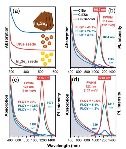
Fig. 5 Absorption spectra of  $In_2Se_3$  seeds, CIS seeds, and  $In_2Se_3$  nanosheets (a). Absorption and PL spectra of CISe, CZISe, and core/shell CZISe/ZnS NCs of three different sizes (small, medium, and large CZISe NCs - 8.7 nm, 16.2 nm, and 20.5 nm, respectively; small, medium, and large CZISe/ZnS NCs - 10.9 nm, 18.3 nm, and 22.9 nm, respectively), emitting with PL maxima at 1082 nm (b), 1175 nm (c), and 1218 nm (d) with corresponding PLQY and FWHM values.
