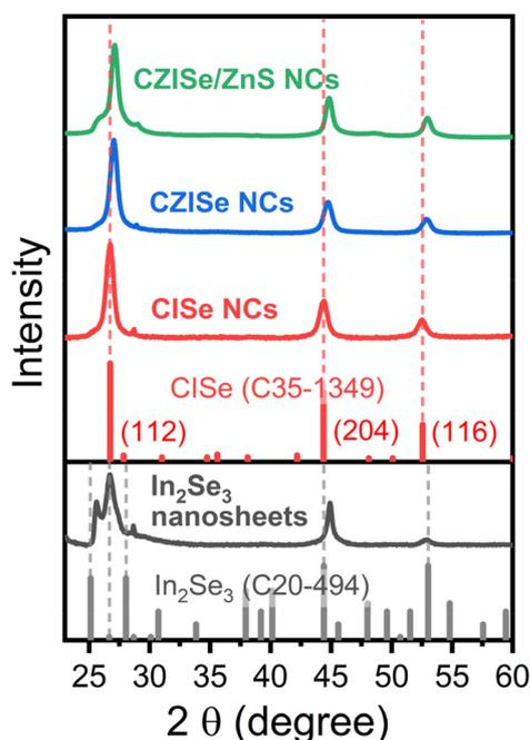
Fig. 2 XRD patterns of  $\text{In}_2\text{Se}_3$  nanosheets, CISE, CZISE, and core/shell CZISE/ZnS NCs with corresponding bulk reference structures of CISE (C35-1349) and  $\text{In}_2\text{Se}_3$  (C20-494) from the JCPDS-ICDD.
