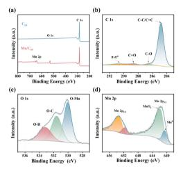
Fig. 3 (a) XPS survey spectrum of Mn/C<sub>60</sub>, and high-resolution XPS spectra of (b) C 1s, (c) O 1s, and (d) Mn 2p.
