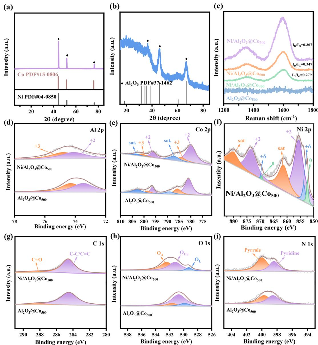
Fig. 2 Wide-angle XRD patterns of (a) Ni/AlOOH@Co<sub>500</sub> and (b) AlOOH@Co<sub>500</sub>. (c) Raman spectra of Ni/AlOOH@Co<sub>600</sub>, Ni/AlOOH@Co<sub>500</sub>, Ni/AlOOH@Co<sub>400</sub> and AlOOH@Co<sub>500</sub> composites. XPS core-level spectra of Al 2p (d), Co 2p (e), Ni 2p (f), C 1s (g), O 1s (h), and N 1s (i) derived from Ni/Al<sub>2</sub>O<sub>3</sub>@Co<sub>500</sub> and Al<sub>2</sub>O<sub>3</sub>@Co<sub>500</sub>.
