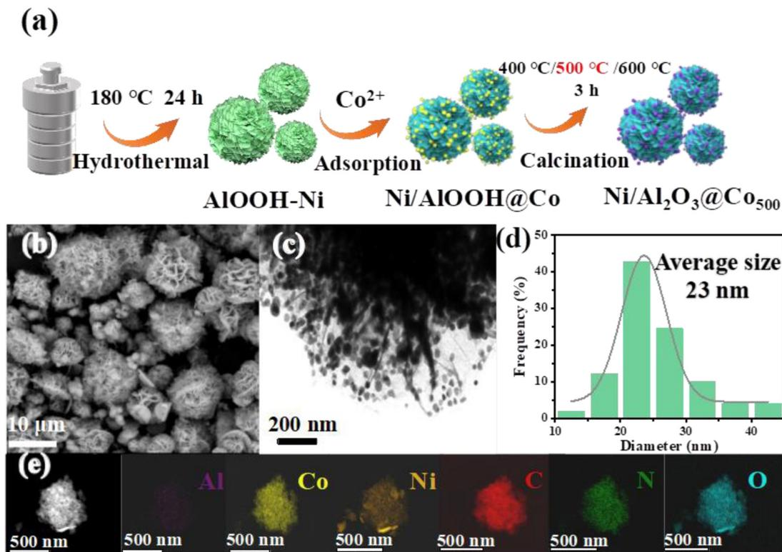
**Fig. 1** (a) Schematic of the synthesis of Ni/Al<sub>2</sub>O<sub>3</sub>@Co<sub>500</sub> catalyst. (b) SEM image, (c) representative TEM image, (d) statistical graph of particle size distribution, and (e) TEM image of Ni/Al<sub>2</sub>O<sub>3</sub>@Co<sub>500</sub> and EDX mapping images of corresponding Al, Co, Ni, C, N, and O elements.
