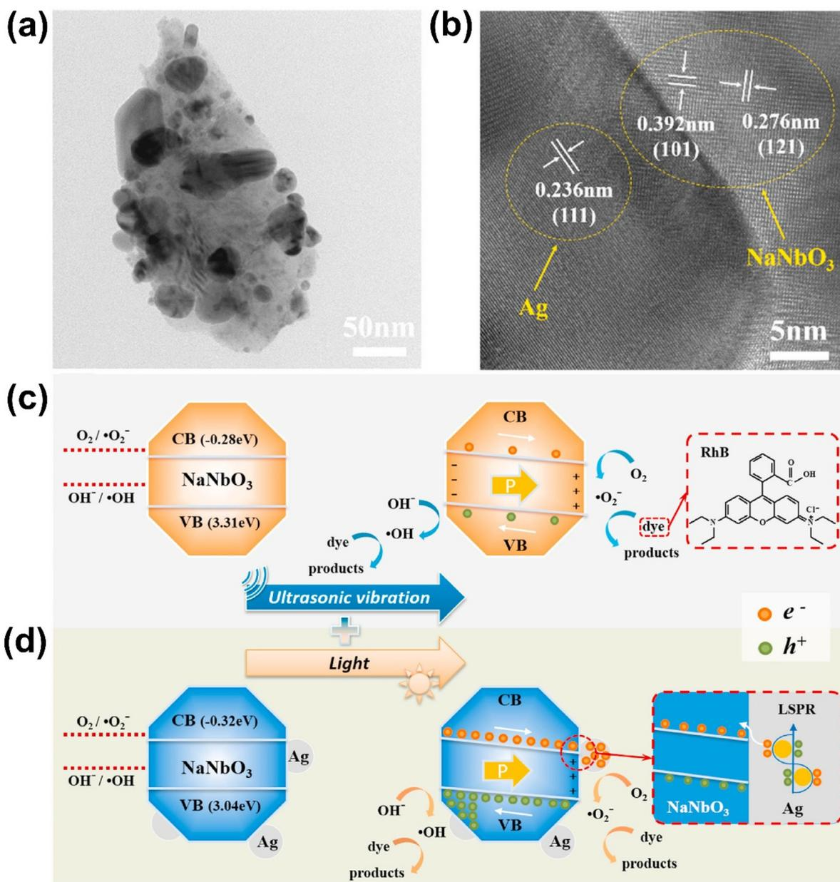
Fig. 11 (a) TEM and (b) HR-TEM images of Ag dot decorated  $\text{NaNbO}_3$ . (c and d) Possible mechanism of piezocatalytic and photo-piezocatalytic dye degradation of Ag/ $\text{NaNbO}_3$ . Reprinted with permission from ref. 133. Copyright 2022, Elsevier.
