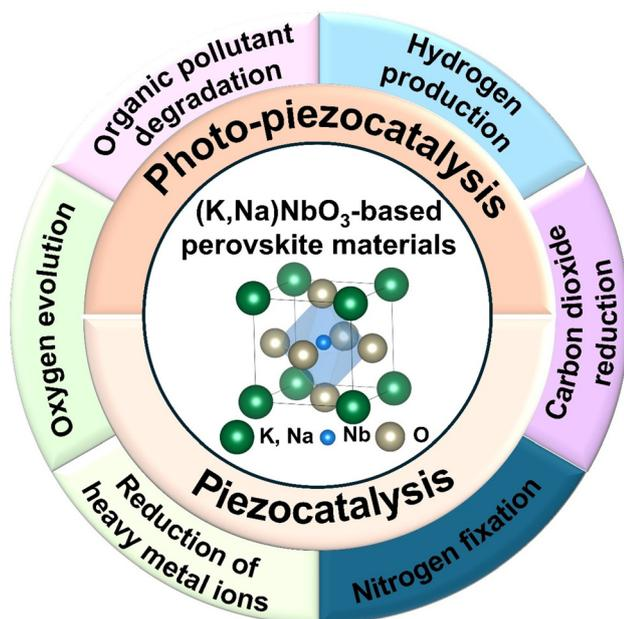
**Scheme 1** Potential application fields of piezocatalysis and photo-piezocatalysis using (K,Na)NbO<sub>3</sub>-based materials.
