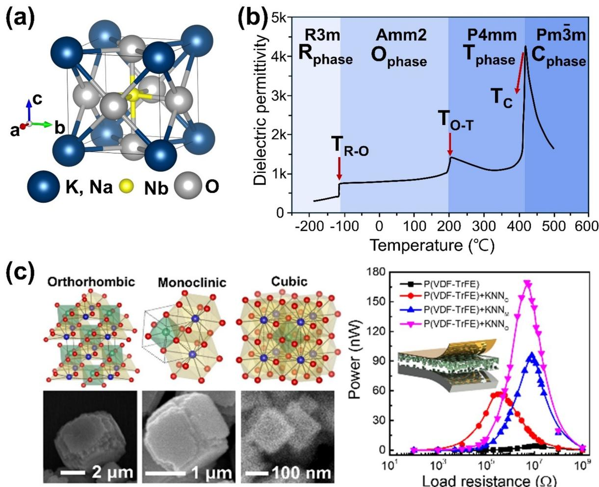
Fig. 1 (a) Crystal structure and (b) temperature-dependent dielectric permittivity of undoped (K,Na)NbO<sub>3</sub> perovskites. (c) Selective phase control of three different phased (K,Na)NbO<sub>3</sub> particles prepared by hydro/solvothermal methods and their corresponding energy harvesting performance. Reprinted with permission from ref. 75. Copyright 2020, American Chemical Society.
