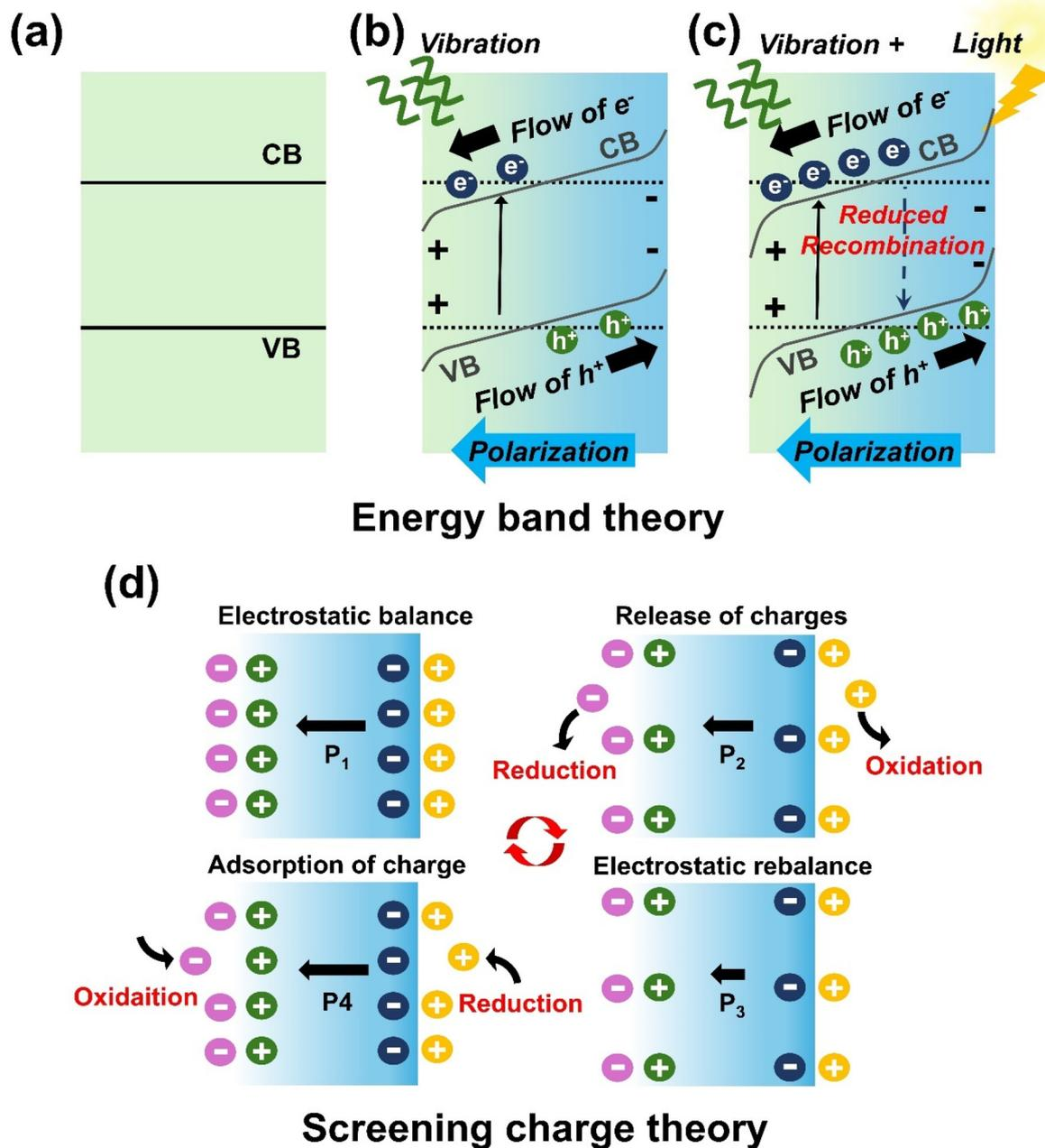
**Fig. 3** Schematic illustrations of energy band structure (a) in the absence of mechanical stimuli (b) under mechanical stress, and (c) under both mechanical and light irradiation. (d) Schematic representation of the screening charge theory showing release and adsorption of surface charges depending on the polarization developed in a piezoelectric material.
