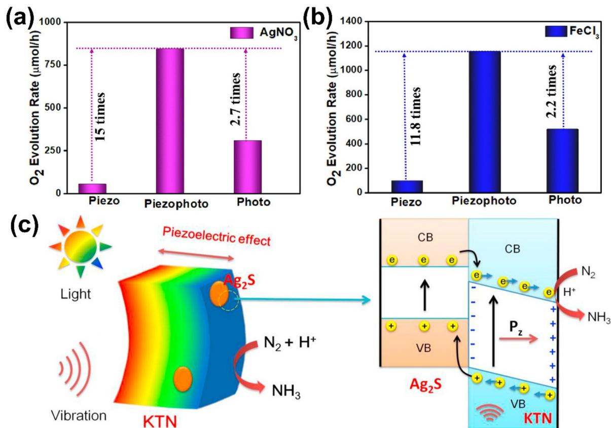
**Fig. 14** (a and b) Photo-piezocatalytic oxygen evolution rates over  $\text{NaNbO}_3/\text{FeOOH}$  in the presence of (a)  $\text{AgNO}_3$  and (b)  $\text{FeCl}_3$  as sacrificial agents. Reprinted with permission from ref. 154. Copyright 2023, American Chemical Society. (c) Schematic illustrations showing the mechanism of photo-piezocatalytic  $\text{N}_2$  fixation over  $\text{Ag}_2\text{S}/\text{KTN}$  heterojunction. Reprinted with permission from ref. 160. Copyright 2023, Elsevier.
