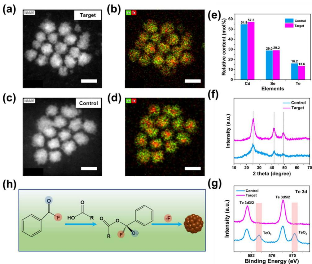
**Fig. 1** (a and c) HAADF-STEM image, (b and d) STEM-EDS mapping of the target and control CdSeTe QDs with and without *in situ* fluorination treatment, respectively. The scale bar is 10 nm. (e) ICP element analysis, (f) XRD, and (g) Te 3d XPS results of the target and control CdSeTe QDs. (h) The possible reaction mechanism of the target CdSeTe QDs with *in situ* fluorination treatment.
