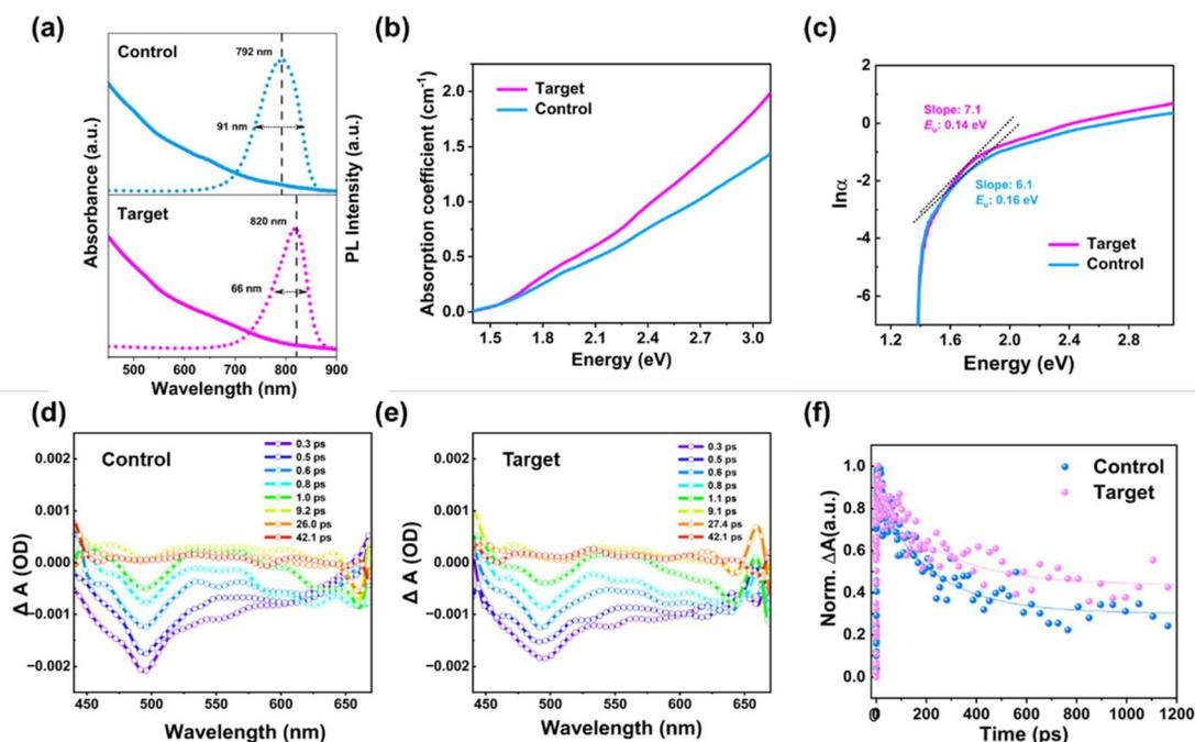
**Fig. 2** (a) The extracted UV-vis and PL emission of the final control and target CdSeTe QDs. (b) Absorption coefficient ( $\alpha$ ) and (c) plot of  $\ln \alpha$  vs. energy used to extract the Urbach energy of the target and control CdSeTe QD films. Ultrafast time-resolved TA spectra of (d) the target and (e) control CdSeTe QDs in toluene. (f) Transient absorption kinetics of the target and control CdSeTe QDs under identical conditions.
