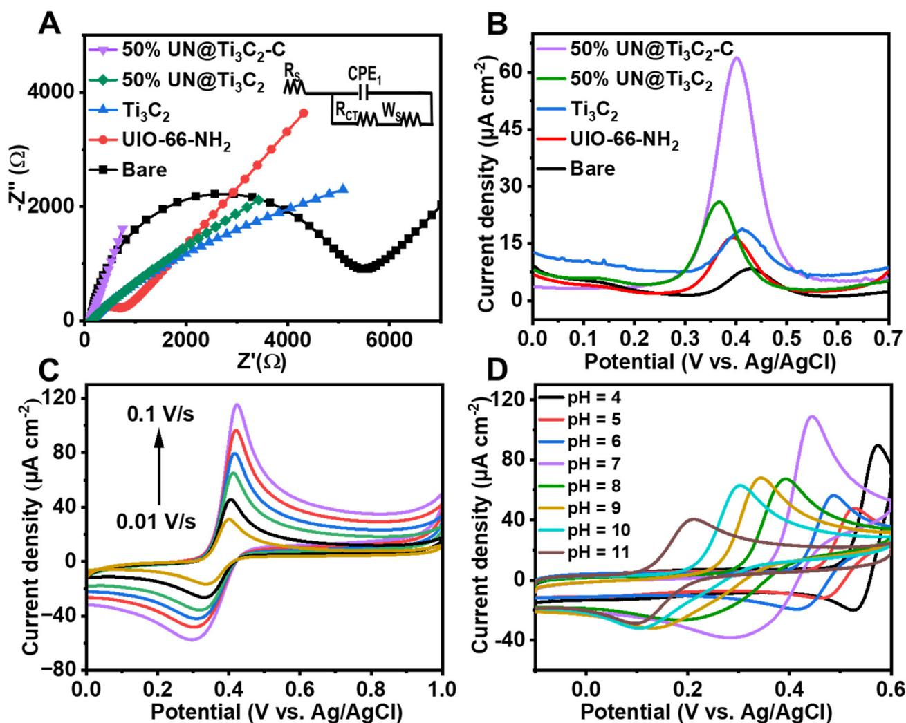
Fig. 4 (A) Nyquist plots of the unmodified and modified electrodes in the 2 mM redox probe of [Fe(CN)<sub>6</sub>]<sup>3-/4-</sup> with 0.1 M KCl, 0.01–10<sup>5</sup> Hz (frequency range). (B) DPV results of various prepared electrodes in 0.1 M PBS with 48 μM AP. (C) Cyclic voltammograms of 50% UN@Ti<sub>3</sub>C<sub>2</sub>-C/GCE at 0.01–0.10 V s<sup>-1</sup> scan rates. (D) Cyclic voltammograms of 50% UN@Ti<sub>3</sub>C<sub>2</sub>-C/GCE in the 48 μM AP solution with various pH.
