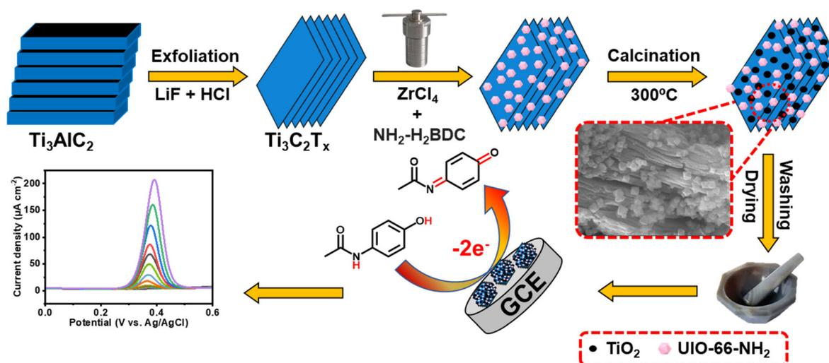
Fig. 1 Schematic diagram of the various steps in UIO-66-NH<sub>2</sub>@Ti<sub>3</sub>C<sub>2</sub>-C synthesis and the electrochemical sensing mechanism.
