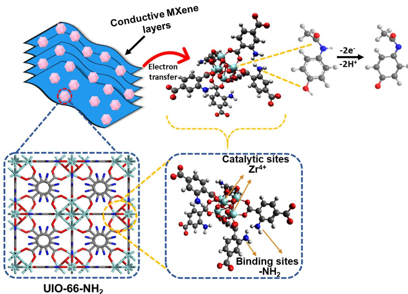
**Fig. 6** Schematic representation of the sensing mechanism for AP using the UN@Ti<sub>3</sub>C<sub>2</sub>-C composite electrode.
