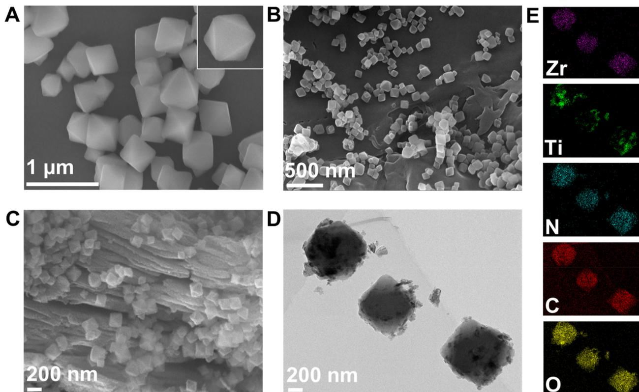
Fig. 2 SEM image of UIO-66-NH<sub>2</sub> (A), UN@Ti<sub>3</sub>C<sub>2</sub> (B), 50% UN@Ti<sub>3</sub>C<sub>2</sub>-C (C), TEM image of 50% UN@Ti<sub>3</sub>C<sub>2</sub>-C (D), the corresponding elemental mapping of 50% UN@Ti<sub>3</sub>C<sub>2</sub>-C (E).
