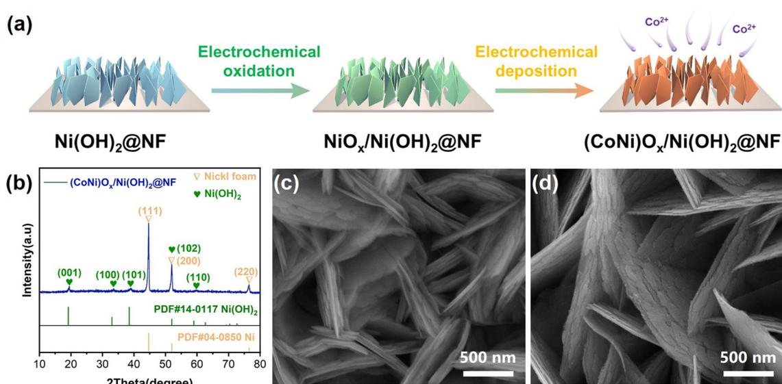
**Fig. 1** (a) Schematic illustration of the preparation process of bimetallic oxy-hydroxides on  $\text{Ni(OH)}_2$  nanosheets. (b) XRD pattern of  $(\text{CoNi})\text{O}_x/\text{Ni(OH)}_2@NF$ . SEM images: (c)  $\text{NiO}_x/\text{Ni(OH)}_2@NF$ , and (d)  $(\text{CoNi})\text{O}_x/\text{Ni(OH)}_2@NF$ .
