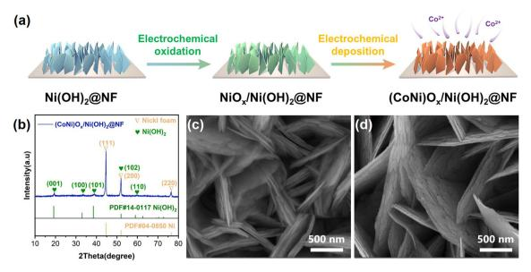
Fig. 1 (a) Schematic illustration of the preparation process of bimetallic oxy-hydroxides on Ni(OH)<sub>2</sub> nanosheets. (b) XRD pattern of (CoNi)O<sub>x</sub>/Ni (OH)2@NF. SEM images: (c) NiOx/Ni(OH)2@NF, and (d) (CoNi)Ox/Ni(OH)2@NF.
