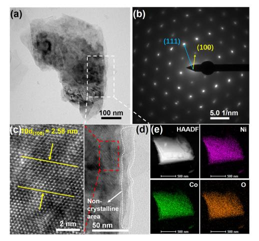
Fig. 2 (a) TEM image of  $(CoNi)O_x/Ni(OH)_2@NF$ . (b) SAED pattern of the core area of  $(CoNi)O_x/Ni(OH)_2@NF$ . (c) High-resolution TEM image of the core area of  $(CoNi)O_x/Ni(OH)_2@NF$ . (e) HAADF and elemental mappings of  $(CoNi)O_x/Ni(OH)_2@NF$ . (e) HAADF and elemental mappings of  $(CoNi)O_x/Ni(OH)_2@NF$ .
