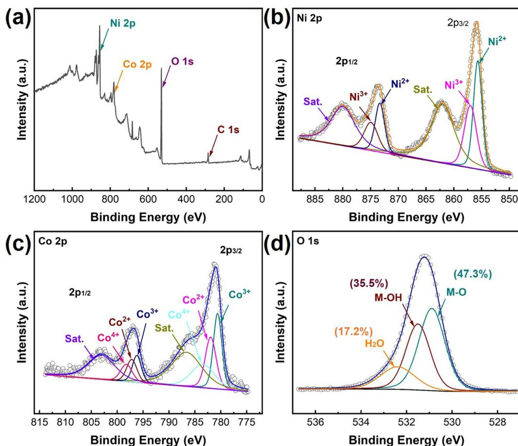
Fig. 3 (a) Survey spectra of (CoNi)<sub>x</sub>/Ni(OH)<sub>2</sub>@NF. High-resolution XPS spectra: (b) Ni 2p, (c) Co 2p, and (d) O 1s.
