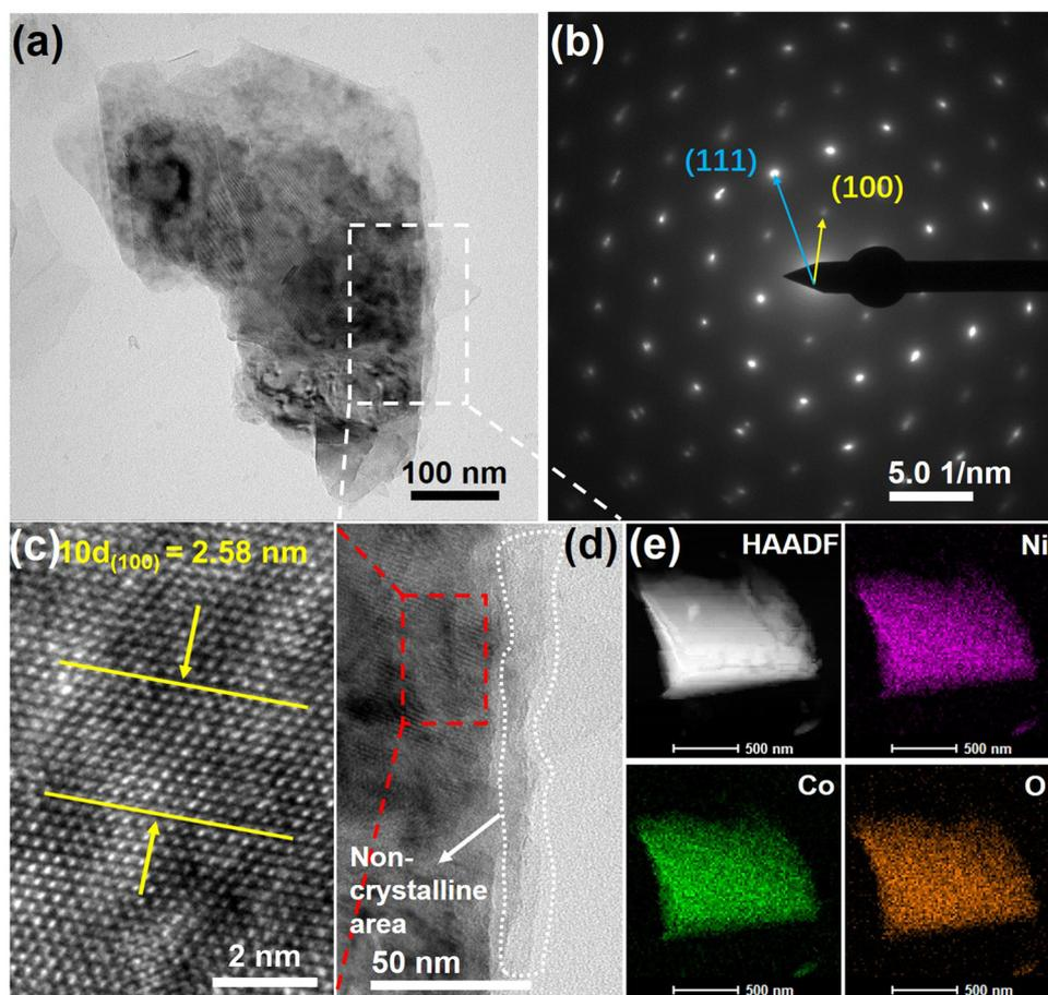
**Fig. 2** (a) TEM image of  $(\text{CoNi})\text{O}_x/\text{Ni}(\text{OH})_2@\text{NF}$ . (b) SAED pattern of the core area of  $(\text{CoNi})\text{O}_x/\text{Ni}(\text{OH})_2@\text{NF}$ . (c) High-resolution TEM image of the core area of  $(\text{CoNi})\text{O}_x/\text{Ni}(\text{OH})_2@\text{NF}$ . (d) TEM image of the rim area of  $(\text{CoNi})\text{O}_x/\text{Ni}(\text{OH})_2@\text{NF}$ . (e) HAADF and elemental mappings of  $(\text{CoNi})\text{O}_x/\text{Ni}(\text{OH})_2@\text{NF}$ .
