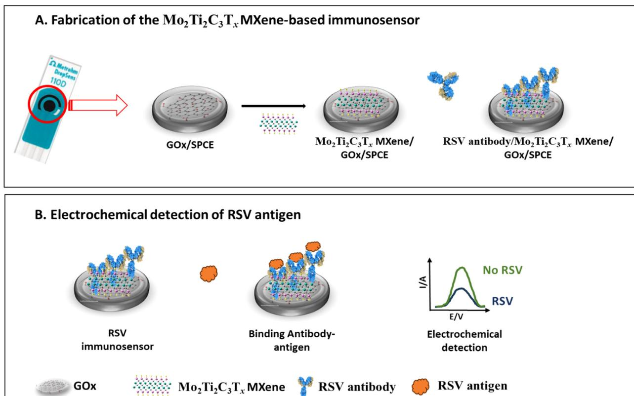
**Scheme 1** Schematic illustration of (A) the fabrication steps of the  $\text{Mo}_2\text{Ti}_2\text{C}_3\text{T}_x$  MXene-based immunosensor and (B) its application in the electrochemical detection of the RSV antigen.
