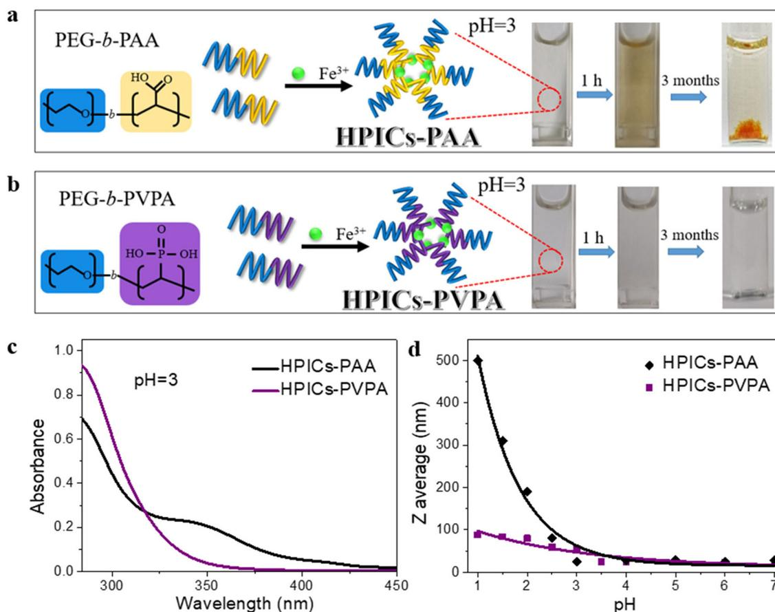
**Fig. 1** (a) Formation of HPICs-PAA and (b) HPICs-PVPA. Aspect of their solutions at different time (0 h, 1 h, 3 months).  $R = 1.0$ . Concentration of Fe is  $1.8 \times 10^{-3} \text{ mol L}^{-1}$  and pH = 3. (c) UV-Vis spectra of HPICs-PAA and HPICs-PVPA solutions (after 1 h). (d) Z-Average diameter of the colloids in solution depending on pH and polymer structure.
