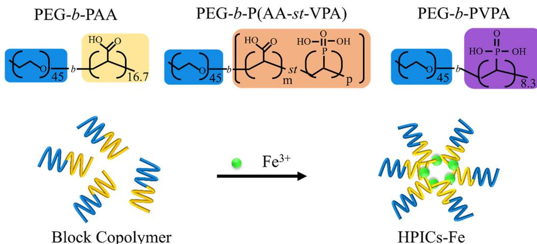
**Scheme 1** Chemical structure of the DHBCs comprising acrylic acid and vinylphosphonic acid as complexing units and schematic representation of HPICs formation by using Fe<sup>3+</sup> to different DHBCs. The indicated values represent the number of repetition units and for PEG<sub>45</sub>-*b*-P(AA<sub>*m*</sub>-*stat*-VPA<sub>*n*</sub>), *m/n* takes the different values 9.3/3.6; 5.6/5.2; 2.5/5.3 (see also Table 2).
