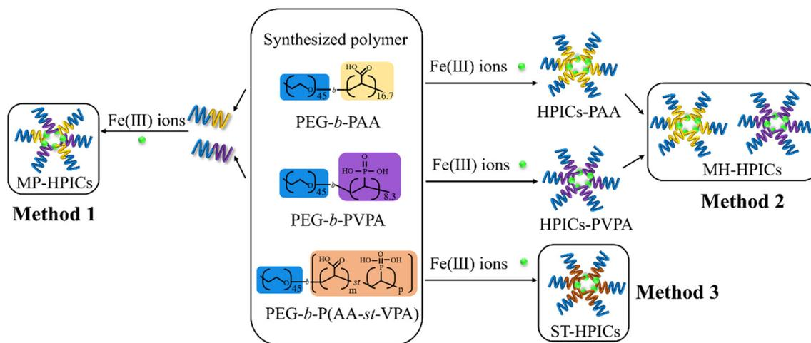
**Scheme 2** Schematic diagram of HPICs samples obtained using three different methods to mix DHBCs containing acrylic acid and vinylphosphonic acid as complexing units. Method 1: HPICs formed from a mixture of polymers (samples denoted MP-HPICs). Method 2: mixing of pristine HPICs (samples denoted MH-HPICs). Method 3: HPICs formed from a block-Statistical copolymer (samples denoted ST-HPICs).
