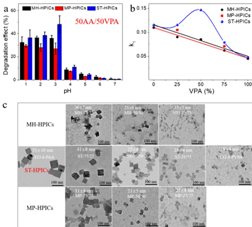
**Fig. 4** Comparison of the properties of ST-HPICs, MH-HPICs and MP-HPICs. (a) Photo-Fenton degradation of AB1: conversion at different pHs for a constant 50/50 AA/VPA ratio. (b) Prussian blue formation: evolution of rate constants  $k_1$  as a function of VPA content for the three families of colloidal structures. (c) TEM images of obtained PB nanoparticles (pH = 5).
