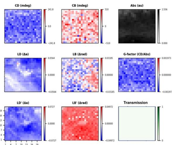
Fig. 5 MMP maps calculated from MM using the analytic inversion method of a spin coated film of ( $S,S$ )-1 at 600 nm of a  $0.5 \times 0.5$  mm area ( $21 \times 21$  steps) with a lateral resolution of 25  $\mu\text{m}$ .
