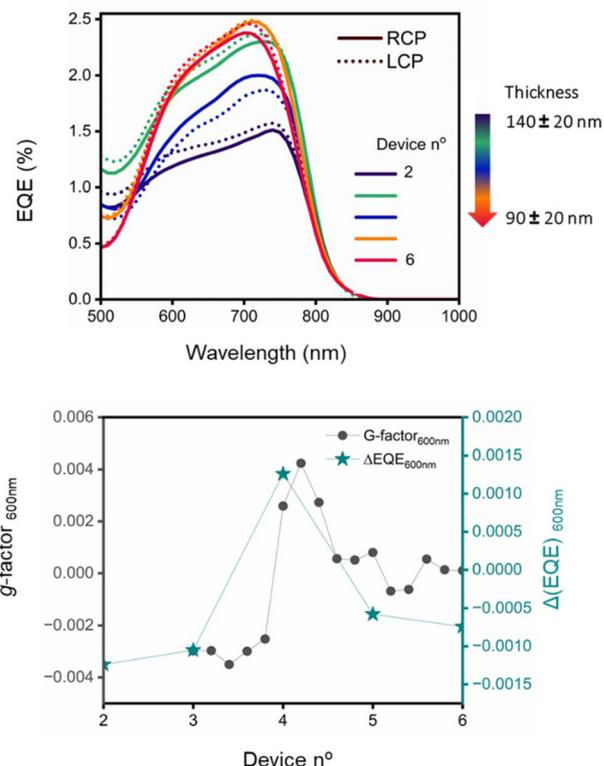
**Fig. 11** (Top) EQE(%) calculated with right (solid line) and left (dotted line) CPL of different devices along the gradient of the cell; (bottom) comparison between the value of  $g$ -factor at 600 nm and the  $\Delta$ (EQE) at 600 nm for the different devices in the gradient cell. To avoid any degradation effects, experiments were systematically performed in the sequence starting with RCP followed by LCP.
