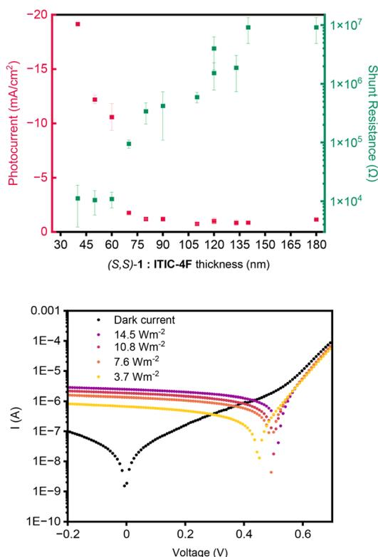
**Fig. 10** Shunt resistance and photocurrent generated under AM 1.5 G illumination for (S,S)-1:ITIC-4F as a function of film thickness in the devices (top) and below the  $J$ - $V$  characteristics of the blend, recorded in the dark and under unpolarized illumination with increasing light intensity.
