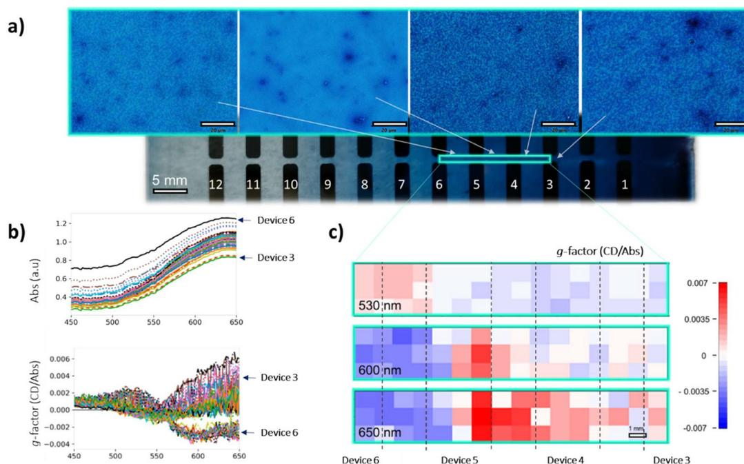
**Fig. 9** (a) Optical micrographs of sections of the solar cell (photograph below) that is made of two rows of 12 devices each of (S,S)-1:ITIC-4F (scale bar of 5 mm). (b) Absorption (top) and apparent *g*-factor (below, from analytic inversion method) spectra measured along the gradient of the solar cell of (S,S)-1:ITIC-4F from 650 nm to 450 nm, in a 16 × 3 grid at 1 mm intervals. (c) 2D maps from apparent *g*-factor values of the spectra at 530, 600, and 650 nm, respectively.
