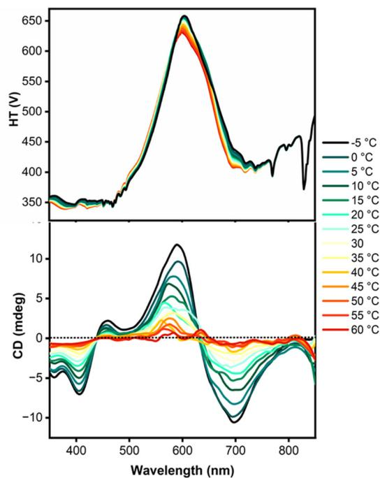
Fig. 2 High-tension (HT, equivalent to absorption, above) and CD (below) spectra at different temperatures for solutions of the enantiomers of (*S,S*)-**1** in chloroform : heptane (1 : 5,  $32 \mu\text{M}$ ) from a commercial spectropolarimeter.
