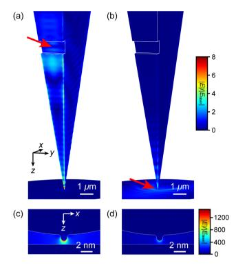
Fig. 5 Distributions of the enhancement factor under groove (a and c) and apex (b and d) illumination at an excitation wavelength of 780 nm. The incident wave vector (red arrow) is in the x-z plane and forms an angle of 35° with respect to the horizontal plane.
