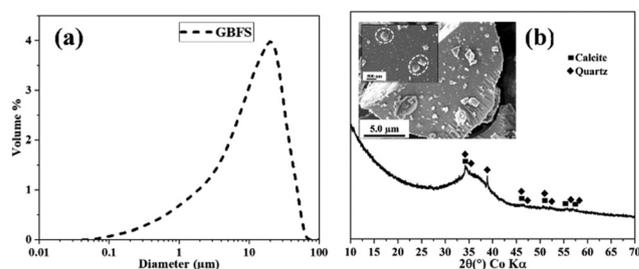
**Fig. 1** (a) PSD of raw GBFS and (b) XRD with SEM images of raw GBFS, where dashed white circles in the enclosed SEM image show the nucleated masses on GBFS particle surface identified as calcite phase which will be discussed in later sections.
