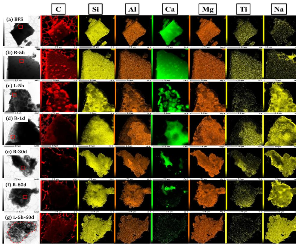
**Fig. 8** TEM-images and elemental mapping of the (a) unreacted GBFS and (b–g) are solids after dissolution experiments for both reference and ligand system. Red squares and dashed red circle in the TEM images are the representative areas analysed with mapping tool (values are presented in Table 2).
