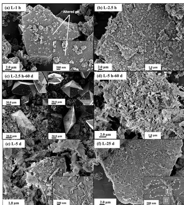
**Fig. 6** SEM images of surface morphology of the GBFS particle and precipitation products (a–f) of the ligand system (L), where the number indicates reaction time in the dissolution experiments in hours (h) or days (d).
