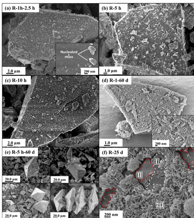
**Fig. 5** SEM images of surface morphology of the GBFS particles and precipitation products (a–f) of the reference system (R), where the number indicates reaction time in the dissolution experiments in hours (h) or days (d).
