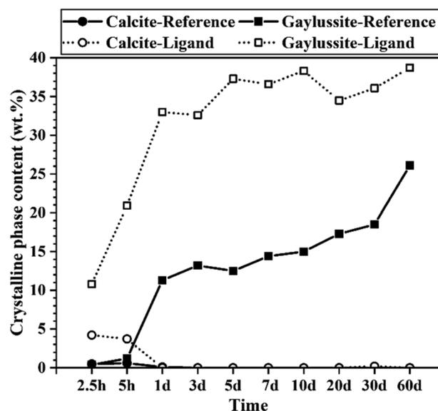
**Fig. 7** Crystalline phase contents based on Q-XRD analysis after respective dissolution reaction times in reference and ligand systems. Natrite was present  $\leq 2$  wt% in both system throughout the reaction time where  $\leq 0.2$  wt% of hydrotalcite was present from 1 d in the reference.
