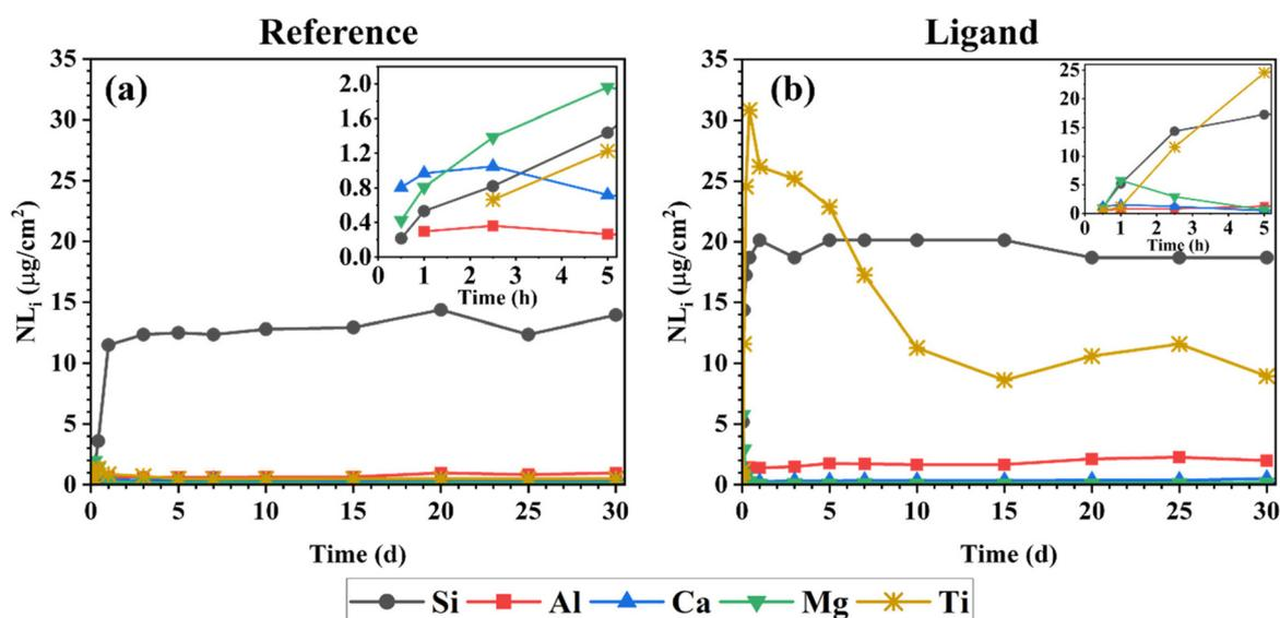
Fig. 3 Normalised mass loss (NLI) versus dissolution time (a) reference (b) ligand (magnified images inside respective graph represents the initial hours of reaction). Based on the replicated dissolution experiments, NLI results had a standard deviation of  $\leq 0.4 \mu\text{g cm}^{-2}$ .
