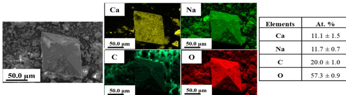
**Fig. 9** Representation of SEM-EDS elemental mapping of gaylussite crystals (left) and averaged SEM-EDS elemental composition of gaylussite crystals (right).  $\pm$  values in the table represent standard deviation.
