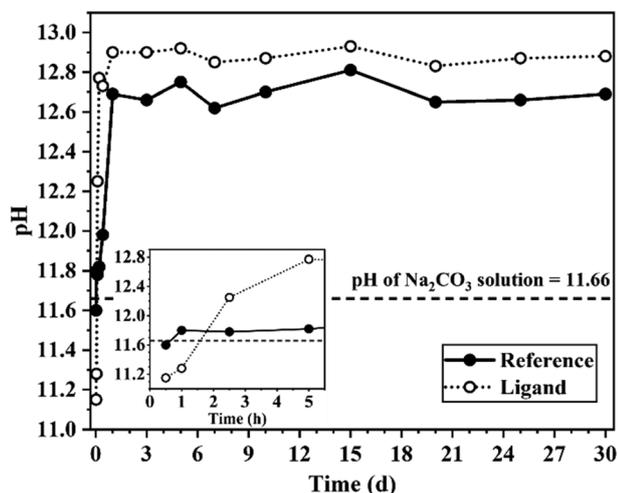
Fig. 2 pH of the solution after respective dissolution time for both reference and ligand system (magnified image inside the graph represents pH in initial hours (until 5 h) of reaction). Replicability of the pH results had a standard deviation of  $\leq 0.032$  pH units.
