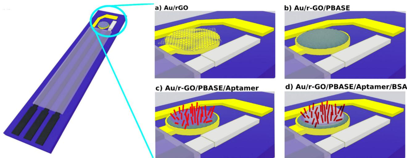
**Fig. 4** (a) Schematic image of the Au electrode deposited on the surface of polyimide (PI). The functionalization of the modified r-GO/PBASE electrode (b) before and (c) after aptamer immobilization and (d) after blocking the surface with BSA is illustrated. Here, the aptamers are presented by red rods.
