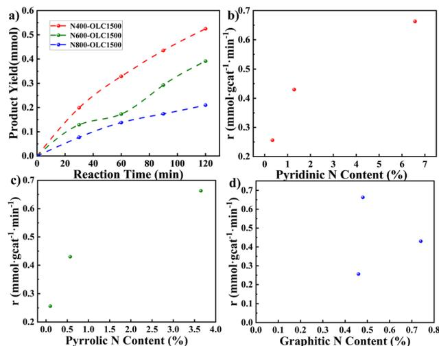
Fig. 5 (a) The change in  $CO_2$  hydroboration product yield with the reaction time (10 mg catalyst, 2 mmol HBpin, 100 °C); (b) the correlation between the initial reaction rate and the pyridinic N content; (c) the correlation between the initial reaction rate and the pyrrolic N content; (d) the correlation between the initial reaction rate and the graphitic N content.
