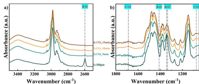
Fig. 6 (a) The *in situ* FTIR spectra of HBpin and CO<sub>2</sub> on NOLC400 in the range of 3500–2500 cm<sup>-1</sup> and (b) 1800–1050 cm<sup>-1</sup>.
