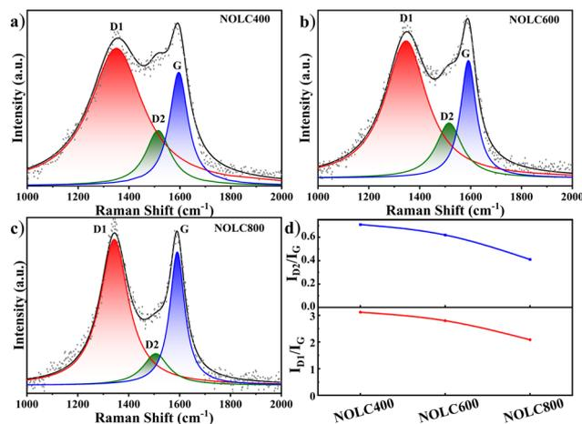
**Fig. 3** (a) The deconvoluted Raman spectra of NOLC400 sample; (b) the deconvoluted Raman spectra of the NOLC600 sample; (c) the deconvoluted Raman spectra of the NOLC800 sample; (d)  $I_{D1}/I_G$  and  $I_{D2}/I_G$  of the NOLCx samples.
