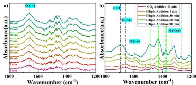
Fig. 7 (a) The *in situ* FTIR spectra of CO<sub>2</sub> adsorption on NOLC400 in the range of 1800–1200 cm<sup>-1</sup>; (b) the *in situ* FTIR spectra of CO<sub>2</sub> reacting with HBpin on NOLC400 (IR peaks marked with green lines result from HBpin).
