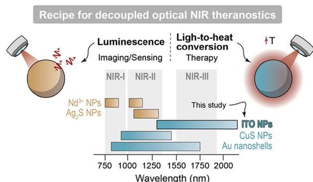
**Fig. 1** Scheme of the aim of this study: filling the void in terms of plasmonic nanoparticles capable of absorbing NIR-III radiation while minimally interfering from an optical standpoint with the NIR-I and NIR-II luminescent nanoparticles. Brown color bars display spectral emission ranges, while blue ones display spectral absorption ranges.
