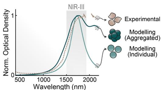
**Fig. 4** Simulated optical response. Comparison between experimentally obtained extinction spectra from ITO NPs in water (brown line) and two modelled extinction spectra in full wave numerical simulations: the modelled extinction spectra of a 7 nm ITO nanosphere (single one, blue line) and an 18 nm agglomeration of spherical ITO NPs (aggregated, dark green) are shown.
